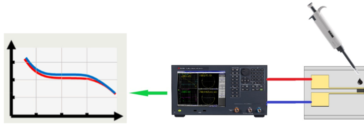
Figure 3.6: Mechanism of electrochemical impedance spectroscopy (EIS) detection.
