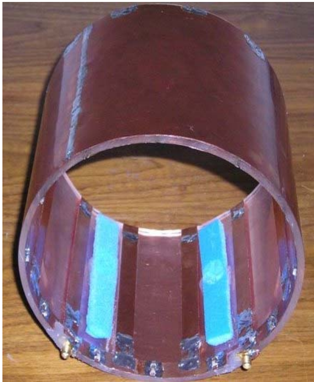
Figure 6.3: A sketch of microstrip based birdcage coil for 1.5 T.
