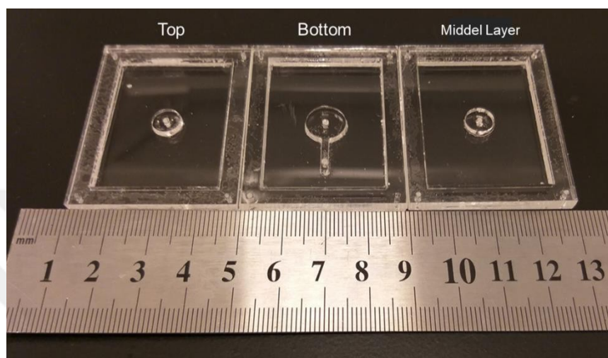
Figure 9 PMMA mold designs for microfluidic chips
