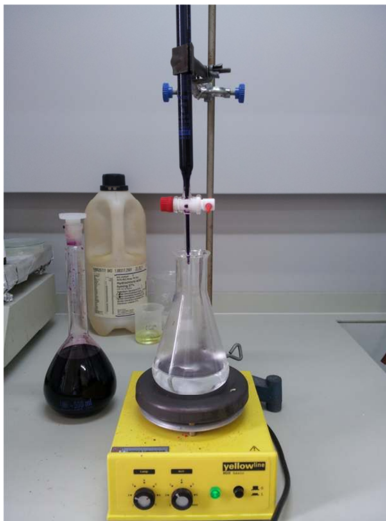
Figure 2.2. A picture of the experimental iodometric titration set-up for determination oxygen stoichiometry.
