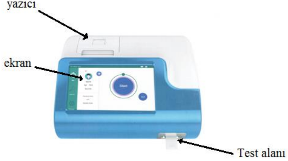
Şekil 16. Getein 1100 immunofluorescence quantitative analyzer
