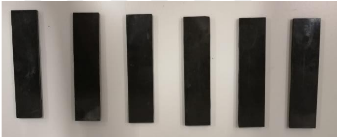
Figure 3.4 Molded final specimens for ultrasonic welding process
