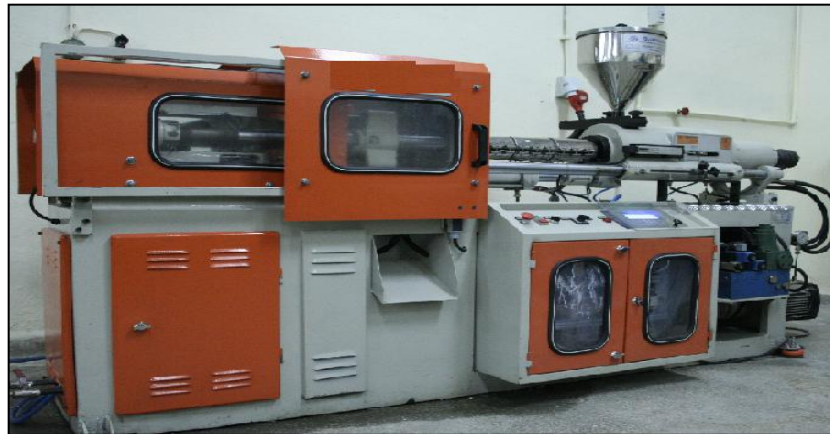
Figure 3.2 40-ton plastic injection machine employed in the experimental study
