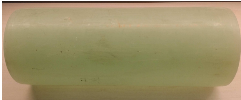
Figure 3.6: Nickel Chloride Hexahydrate solution used as a phantom for imaging.
