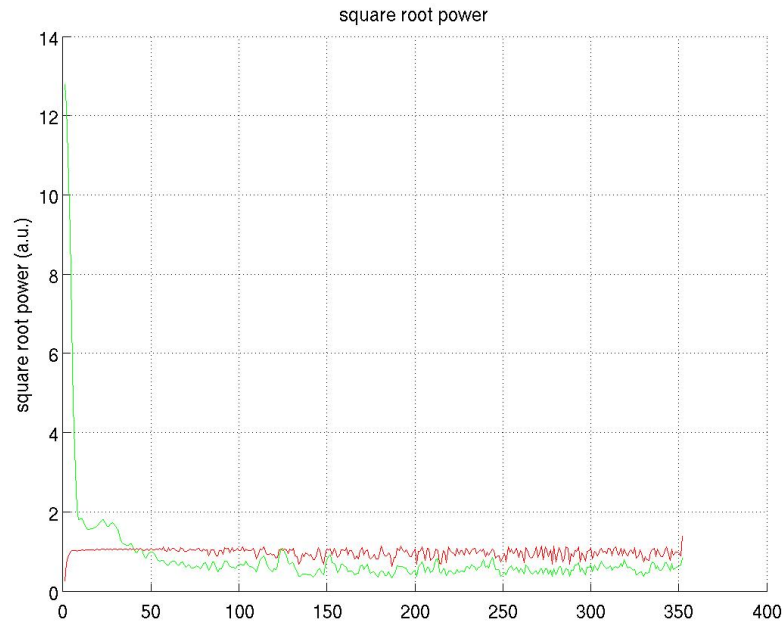
Figure 4.7: Square root power of the currents designed with VERSEp vs k-space samples. Square root power before VERSE optimization (green) and after VERSE optimization (red) are shown.
