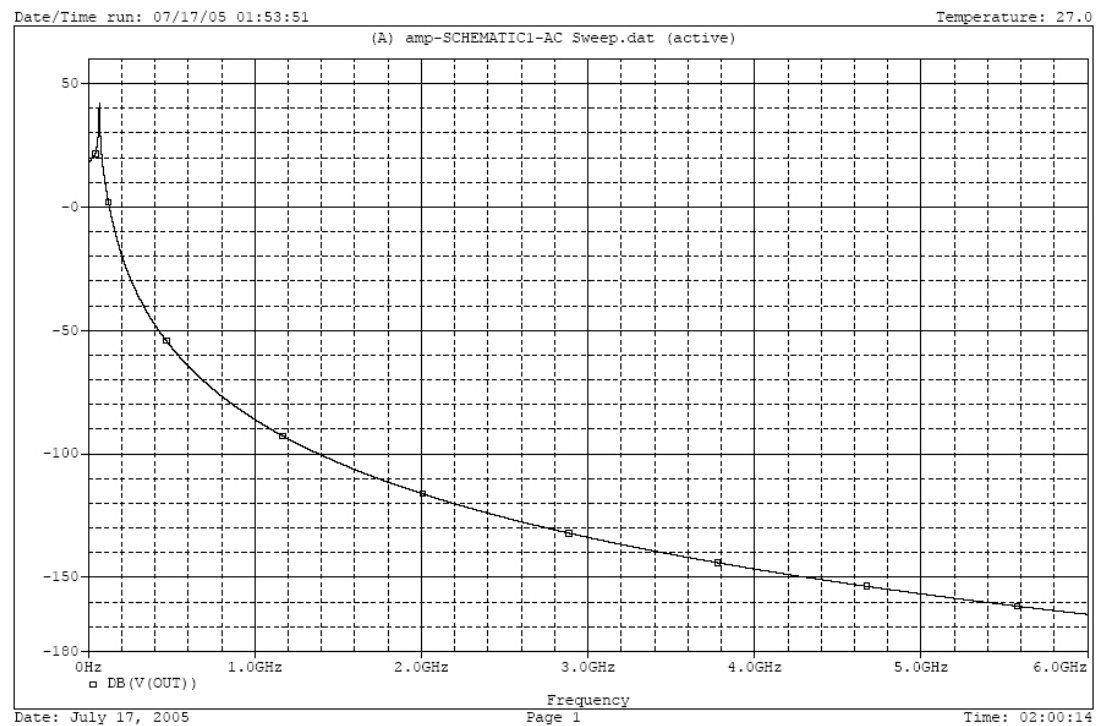
Figure 4.3: AC Sweep by PSpice: Presents the gain of the circuit up to 6Ghz.
