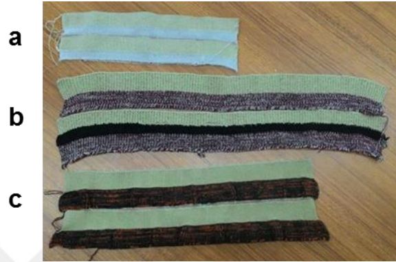
Figure 2.5 The conductive textiles made from the silver thread by (a) the first, (b) the second, and (c) the third weaving technique (Personal archive, 2018)
