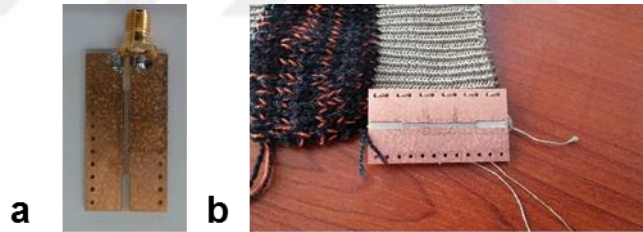
Figure 2.6 (a) Connection circuit. (b) Connection circuit sewn onto the conductive textile (Personal archive, 2018)
