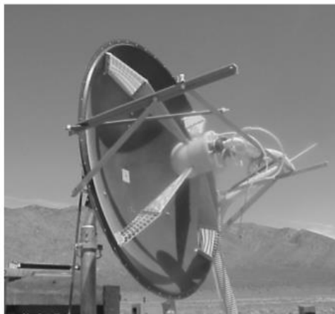
Figure 2.5: An example of a hyperband system with an IRA [16], [17]
