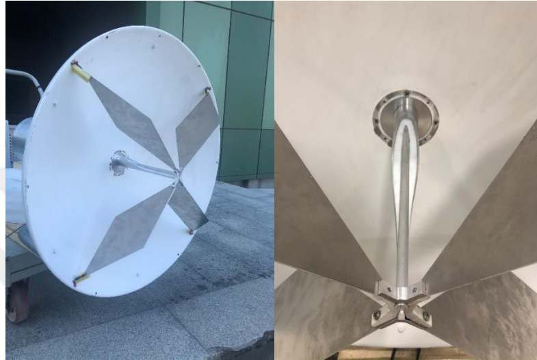
Figure 4.48: Conventional IRA and coaxially tapered balun
