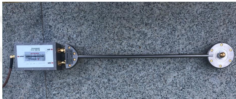
Figure 4.51: D-dot probe manufactured by Montena
