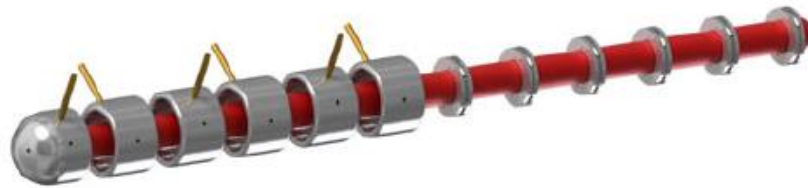
Figure 2.13: Marx generator structure example [24]
