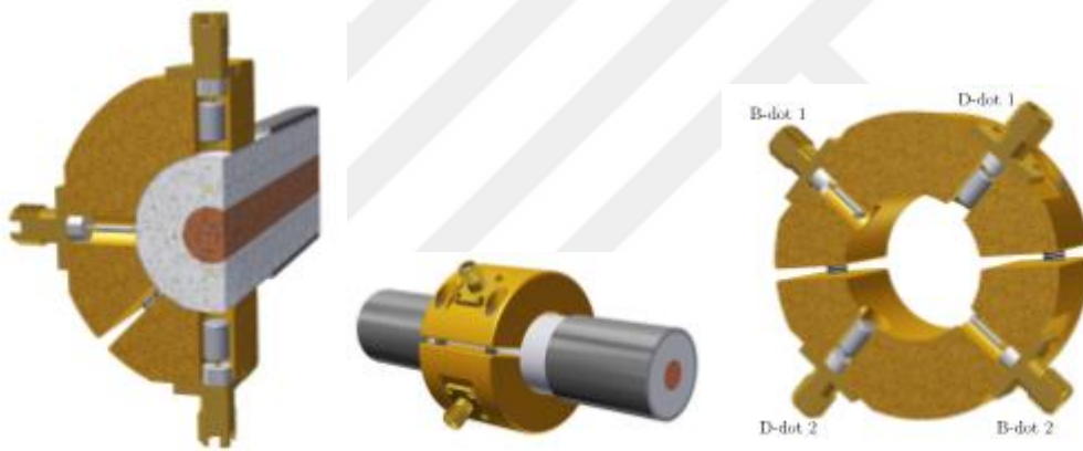
Figure 2.32: D-dot and B-dot probes designed in study [28]
