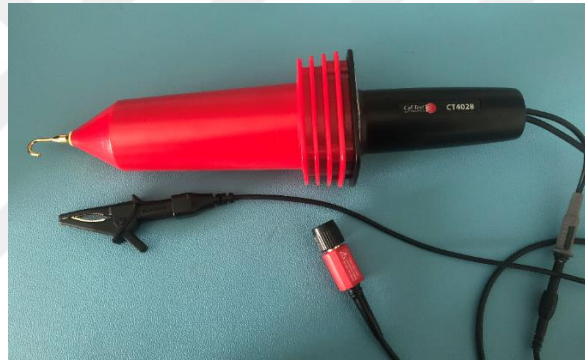
Figure 4.3: Caltest CT4028 39 kV voltage probe
