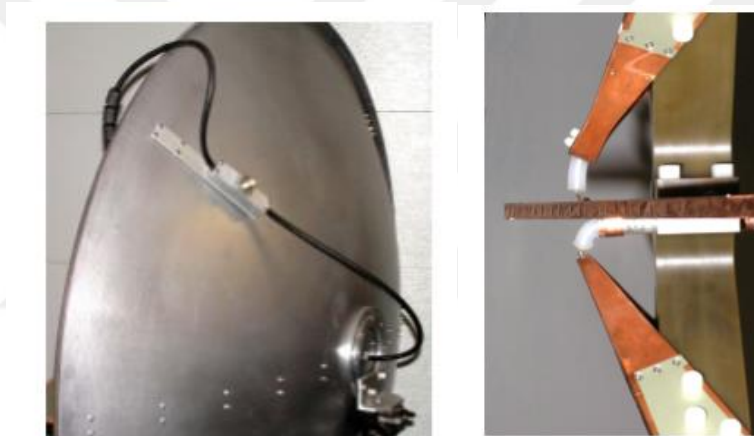
Figure 2.27: Feeding the IRA with splitter balun [43]
