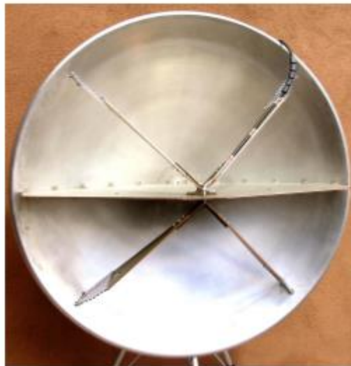
Figure 2.25: An IRA example with 1.52 m diameters [43]
