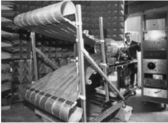
Figure 2.4: H-2 system with a large TEM horn antenna [14]
