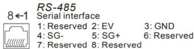
Figure 4.25 RJ45 Ethernet protocol wireframe (DELTA VFD-EL User Manual, 2020)
