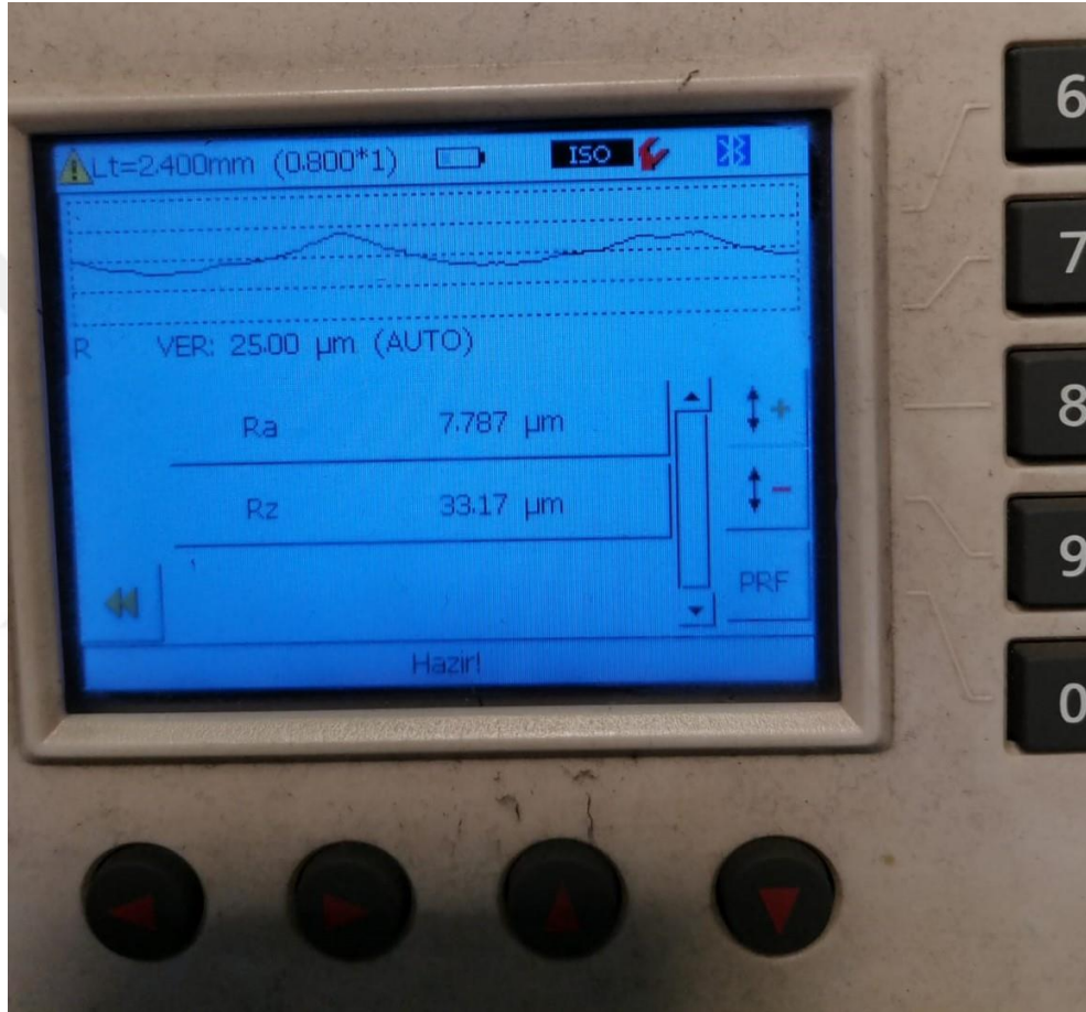
Figure 3.9 Surface roughness values of A2.1 (Personal archive, 2020)
