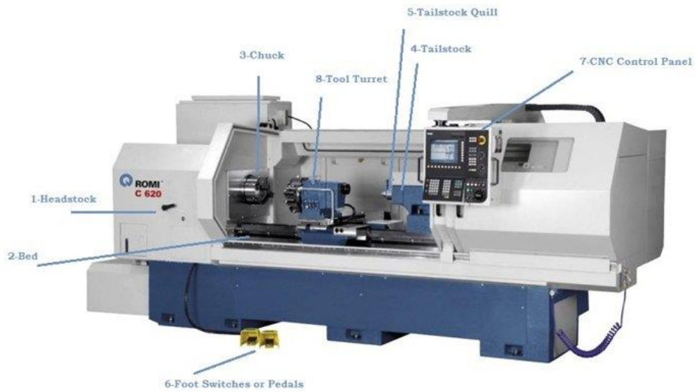
Figure 1.4 View of a modern cnc lathe (Parts of the CNC Lathe, 2020)
