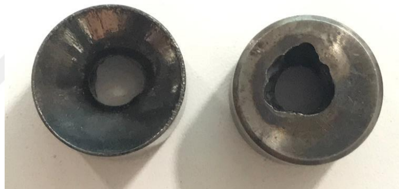
Figure 5.9: Molybdenum Nozzle Insert after 12 sec Burn
