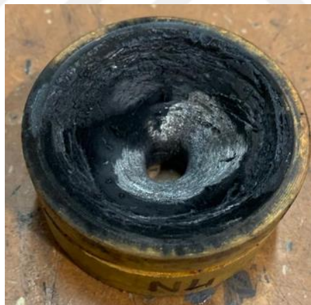
Figure 5.7: Silica Phenolic Nozzle 2 after 12 sec Burn
