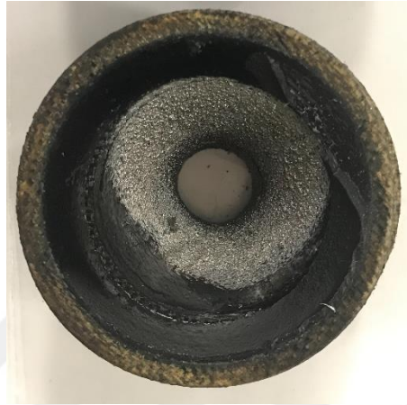
Figure 5.6: Silica Phenolic Nozzle 1 after 12 sec Burn
