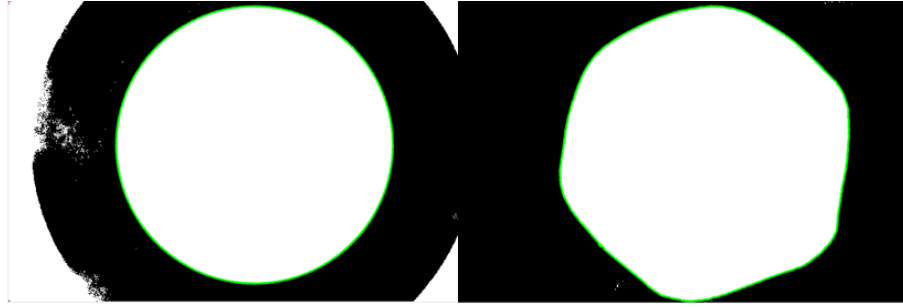
Figure 2.6: Grade 1 Erosion Photos Before and After the Test
