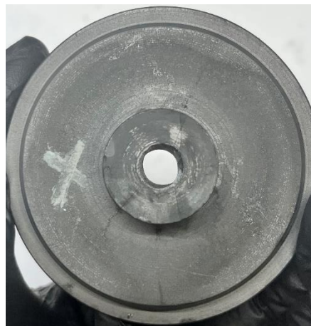
Figure 5.22: Cracks on the Surface of SiC After the Test
