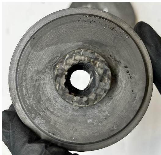
Figure 5.5: C/C Throat Erosion after 12 sec Burn Time
