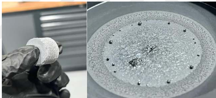
Figure 5.12: Dusty Surface on SiC and Droplets on Crucible
