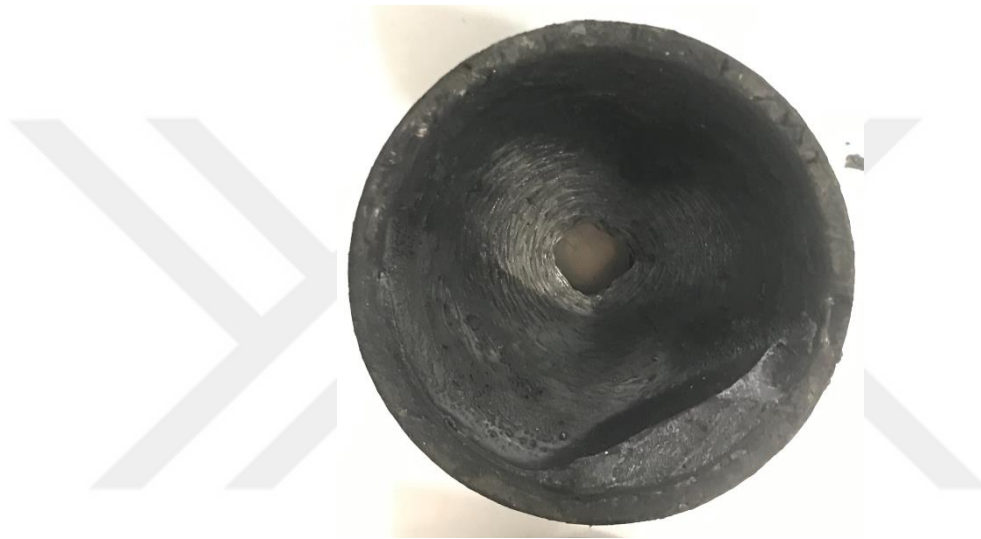
Figure 5.4: Carbon Phenolic1 Throat Erosion after 12 sec Burn
