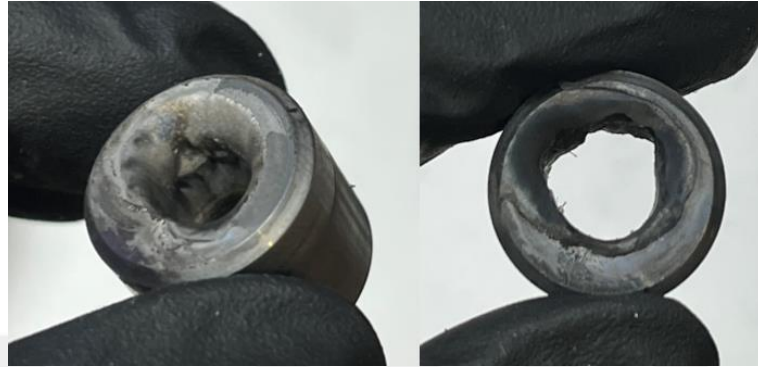
Figure 5.8: Tungsten Nozzle after 12 sec Burn at 2.7 O/F
