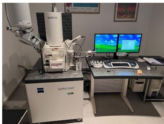
Figure 4.1 Representative scanning electron microscope (SEM) setup, illustrating the instrument layout and control system
