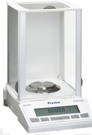
Figure 3.8 High precision microbalance (Precisa XB 220A) used to weigh the MWCNTs and the pristine oils (Precisa, 2016)
