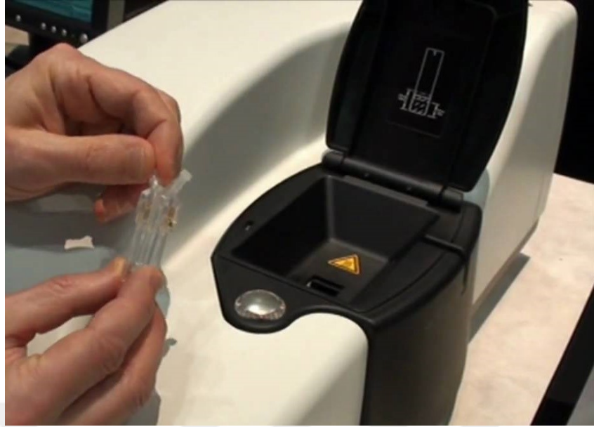
Figure 3.7 Zeta potential and laser particle size analyzer (Zetasizer Nano-ZS) for estimating the particle size distribution with sample holder (DTS1070) (Malvern, 2017)
