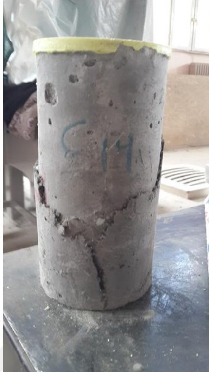
Figure C5 Failure mode of unwrapped ECC specimens exposed to sulfate environment
