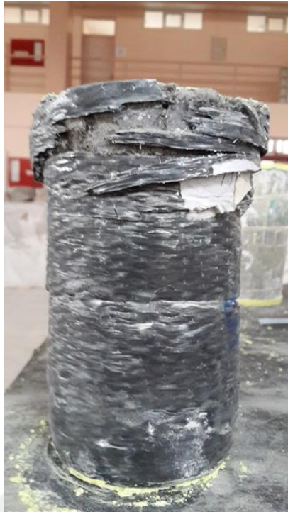
Figure C9 Failure mode of ECC specimens wrapped by CFRP exposed to sulfate environment
