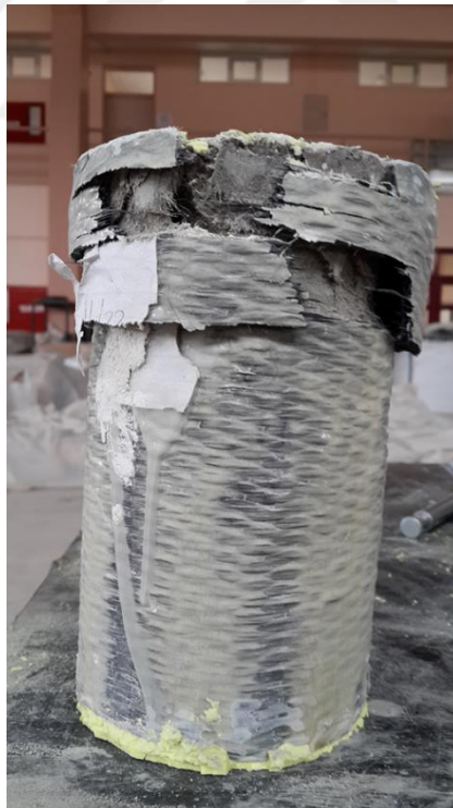
Figure C8 Failure mode of ECC specimens wrapped by CFRP exposed to sulfuric acid environment
