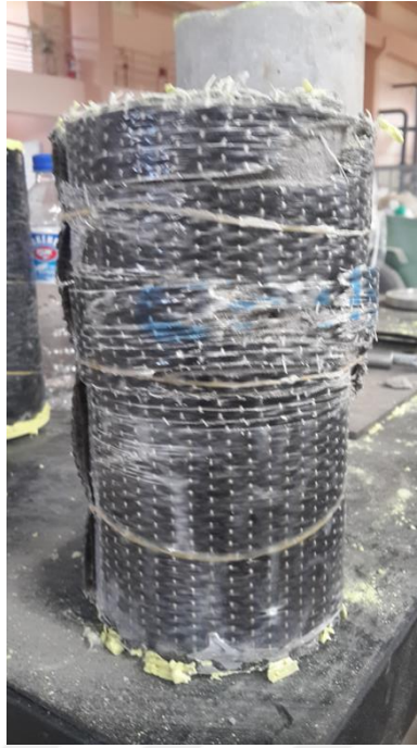
Figure C13 Failure mode of ECC specimens wrapped by BFRP exposed to sulfate environment
