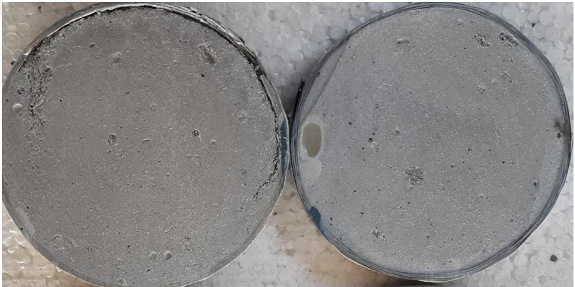
Figure D6 FRP wrapped ECC specimens exposed to acid environment
