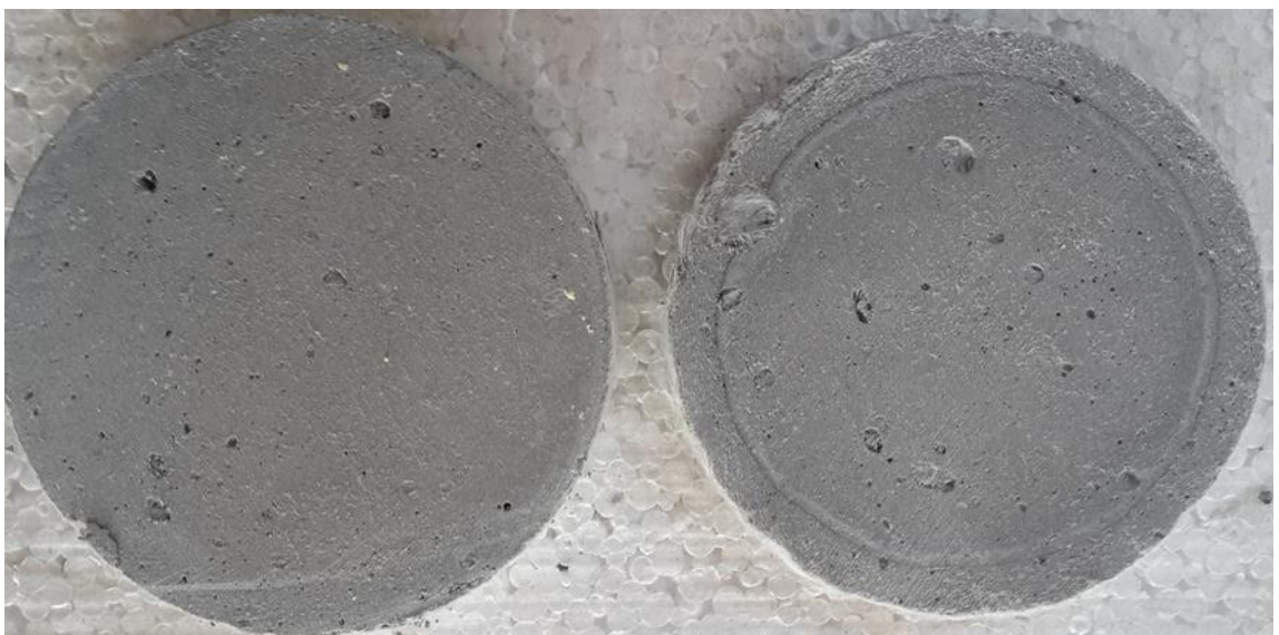
Figure D2 LCFA-ECC specimens exposed to ambient and acid environment
