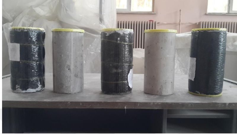
Figure C1 Preparing the ECC specimens for mechanical test
