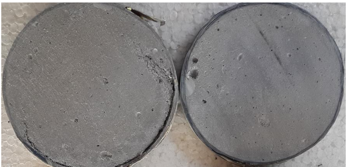
Figure D7 FRP wrapped ECC specimens exposed to sulfate environment
