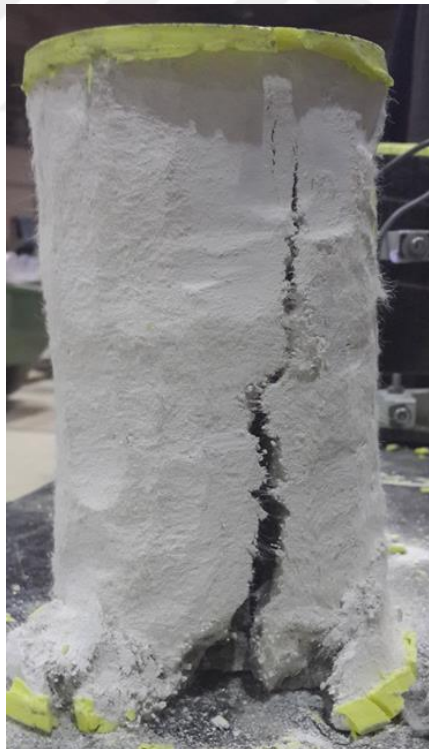
Figure C4 Failure mode of unwrapped ECC specimens exposed to acid environment
