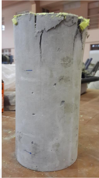
Figure C3 Failure mode of unwrapped ECC specimens exposed to ambient environment
