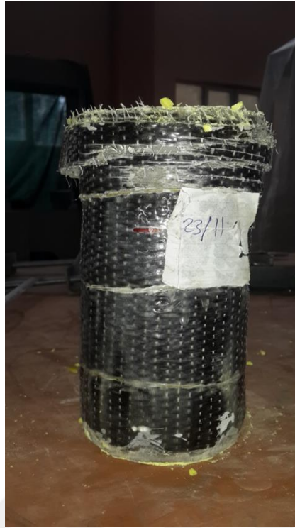
Figure C11 Failure mode of ECC specimens wrapped by BFRP exposed to ambient environment
