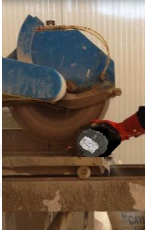
Figure D1 Preparing SEM samples by cutting wrapped and unwrapped ECC specimens
