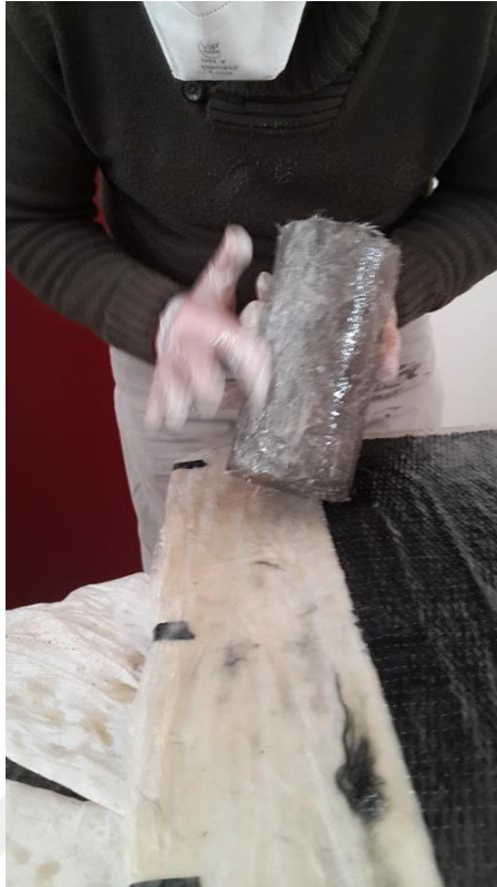
Figure A7 Coating the surface of ECC specimen by epoxy
