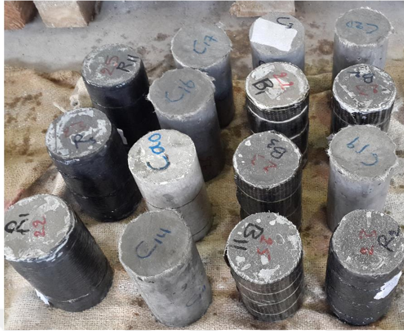
Figure B3 ECC specimens exposed to seawater environment
