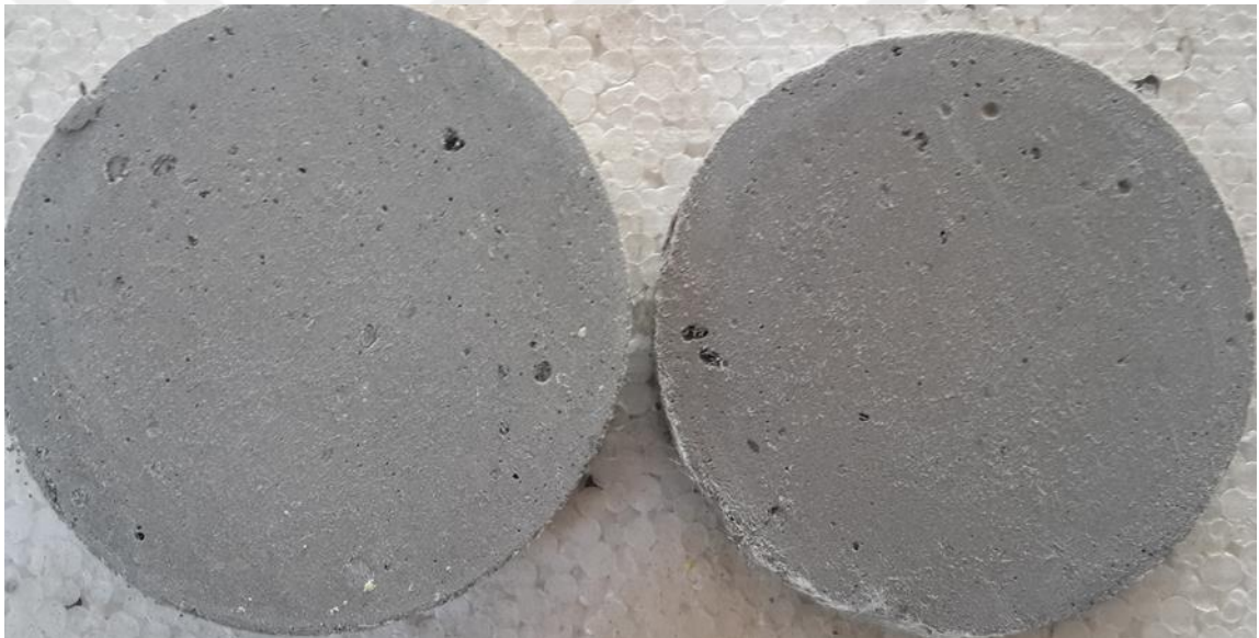
Figure D4 LCFA-ECC specimens exposed to ambient and seawater environment
