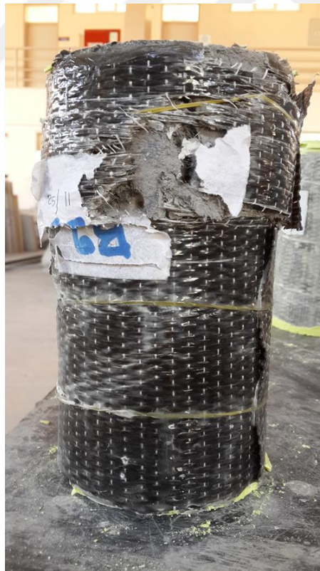
Figure C14 Failure mode of ECC specimens wrapped by BFRP exposed to seawater environment
