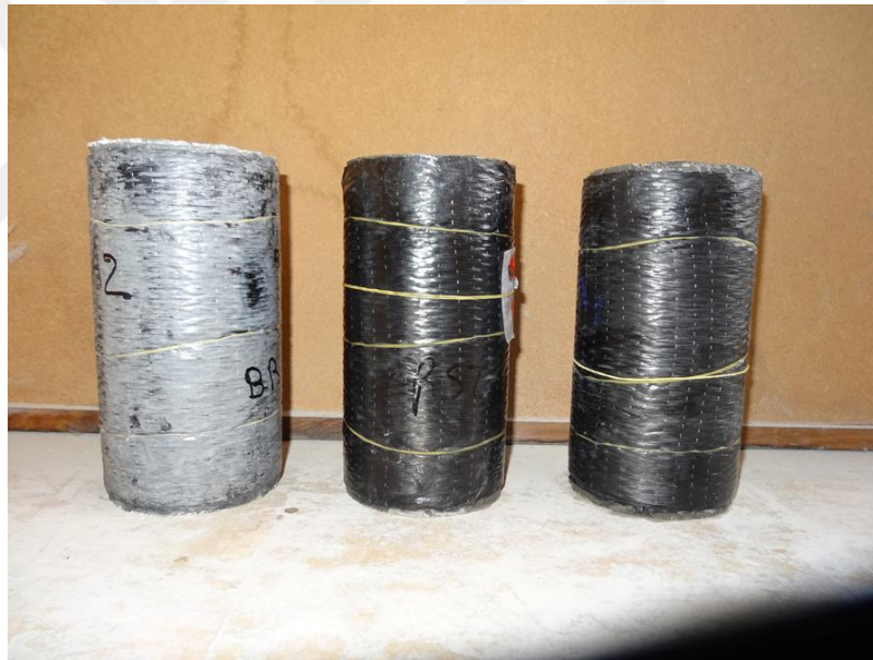
Figure B4 ECC specimens wrapped by CFRP exposed to chemical environment
