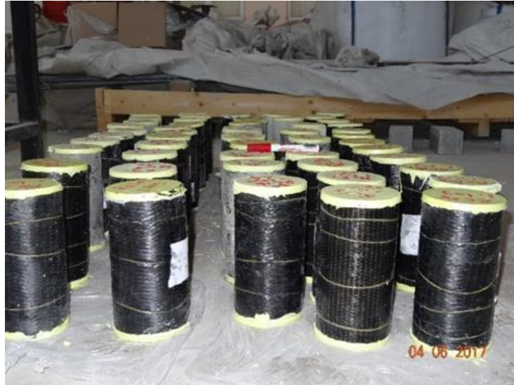
Figure 3.6 Sulfur capped specimens before the uniaxial compression test
