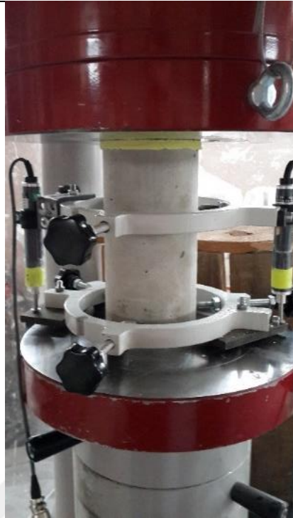
a) Unconfined ECC specimen
