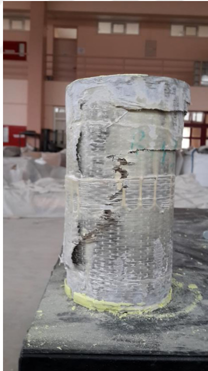
Figure C12 Failure mode of ECC specimens wrapped by BFRP exposed to sulfuric acid environment
