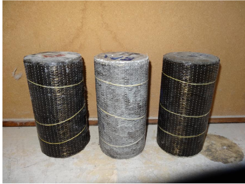
Figure B5 ECC specimens wrapped by BFRP exposed to chemical environment
