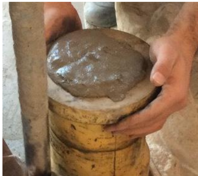
Figure A2 ECC mix vibrated to get proper compacting specimens
