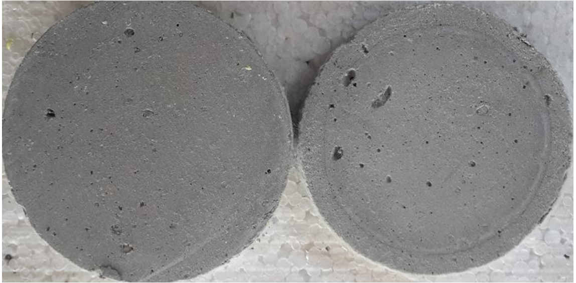
Figure D3 LCFA-ECC specimens exposed to ambient and sulfate environment
