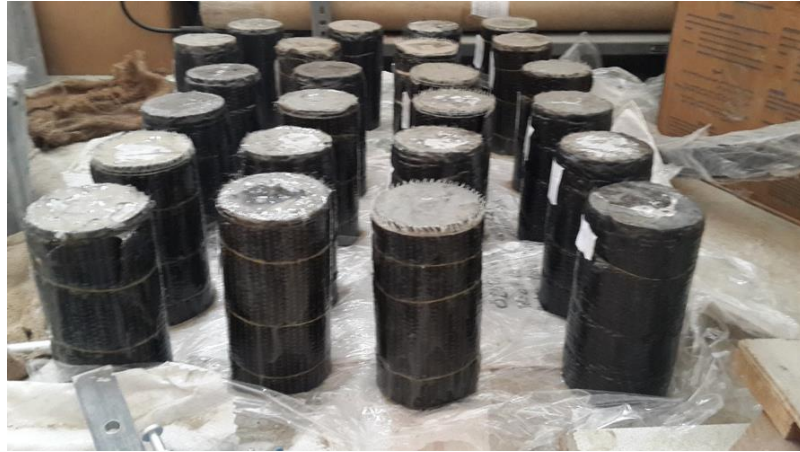
Figure A11 ECC specimens wrapped by FRP fabrics
