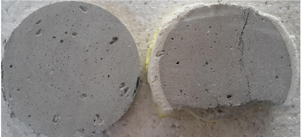
Figure D5 HCFA-ECC specimens exposed to ambient and acid environment
