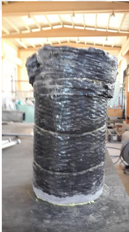
Figure C10 Failure mode of ECC specimens wrapped by CFRP exposed to seawater environment
