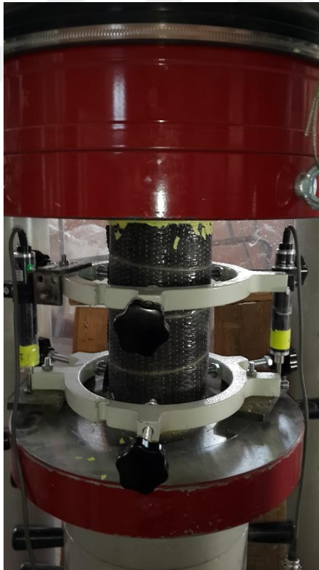
Figure C2 ECC wrapped specimens under axial compression test
