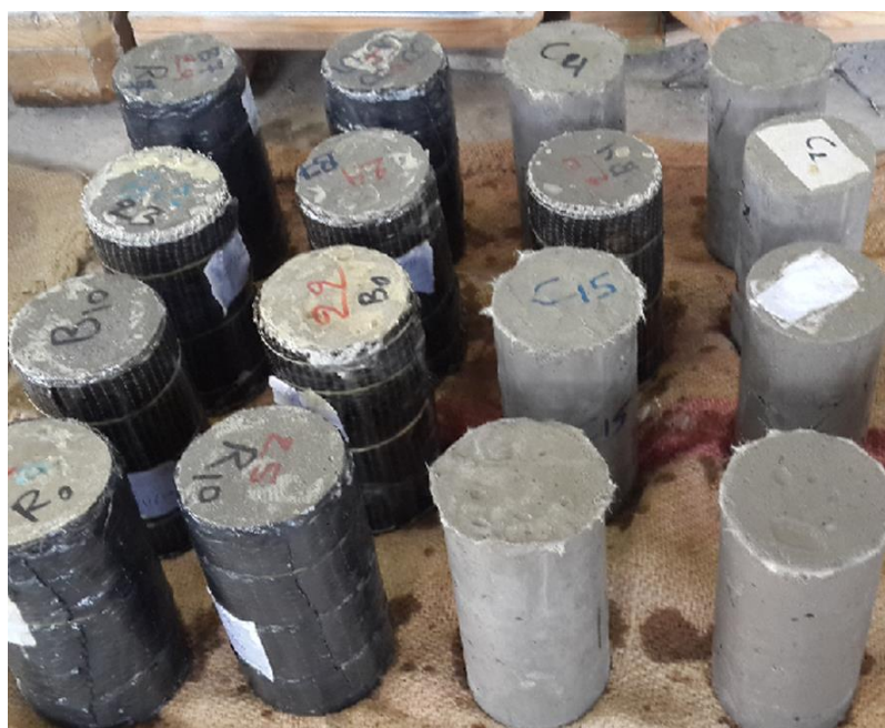
Figure B2 ECC specimens exposed to sulfate environment
