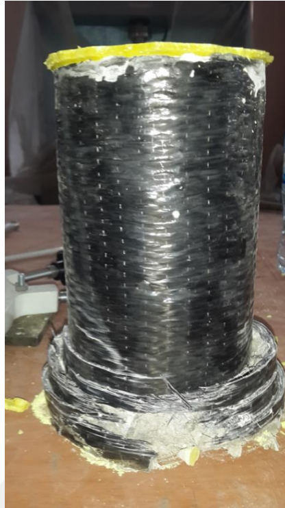
Figure C7 Failure mode of ECC specimens wrapped by CFRP exposed to ambient environment
