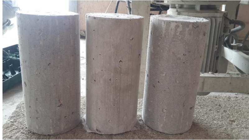
Figure A5 ECC surface prepared and non-prepared specimens
