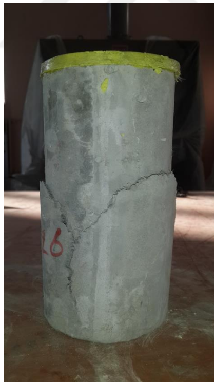
Figure C6 Failure mode of unwrapped ECC specimens exposed to seawater environment
