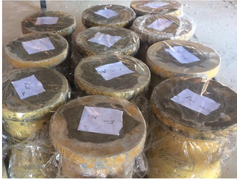
Figure A3 ECC fresh specimens covered by plastic sheet
