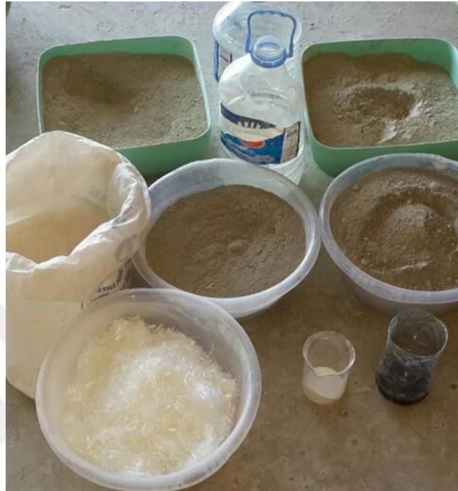
Figure A1 Materials used in the production of ECC specimens
