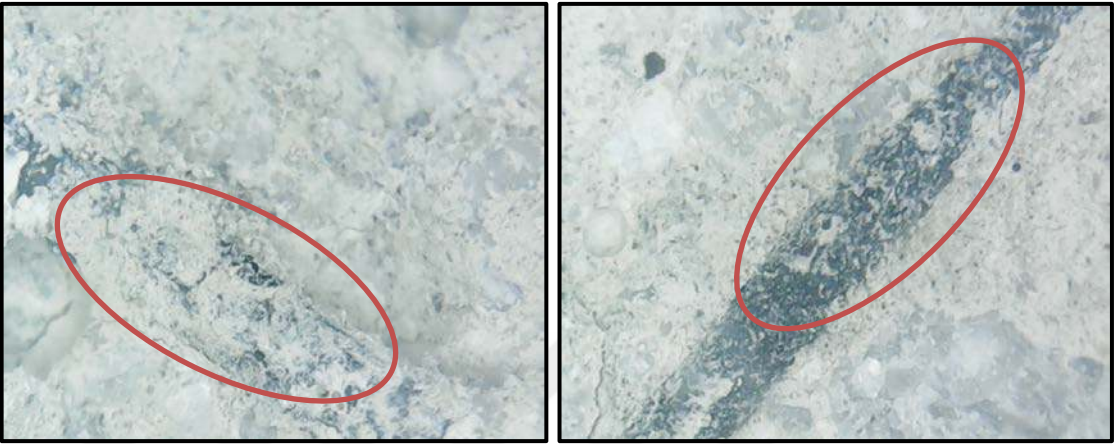
FR-MSCC-S10 mixture FR-HSCC-S10 mixture Figure 4.7 The oxidation and carbonation of SF after exposure to 750°C.
