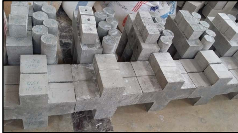
Figure 3.4 Preparing the specimens after curing treatment.
