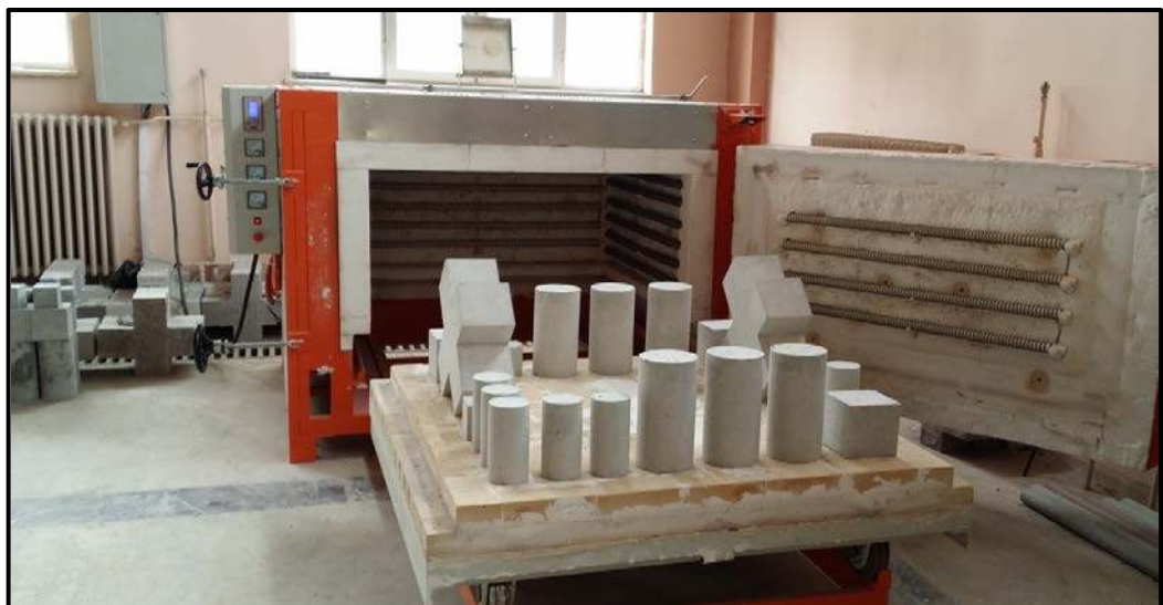
Figure 3.6 Arrangement the specimens inside the electric furnace.
