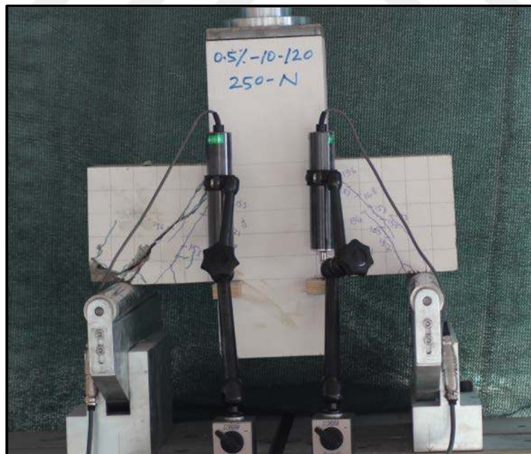
b) Adjusting the LVDT during the testing
