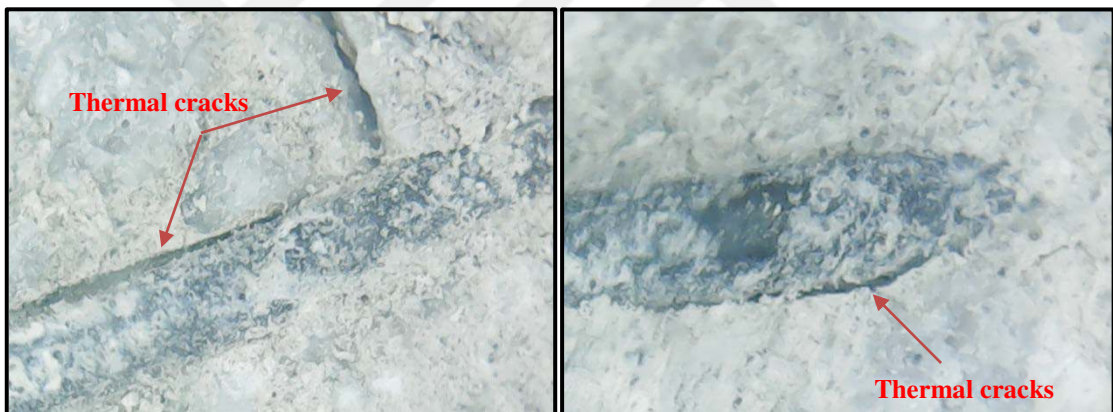
Figure 4.5 Thermal cracks between matrix and SF after exposure to 750°C.
