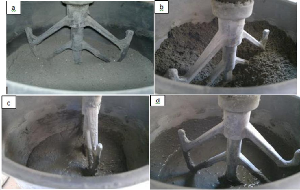
Figure 3.5. Mixing of UHPC: (a) dry mix, (b) water addition, (c) SP addition with low speed, and (d) SP addition with high speed
