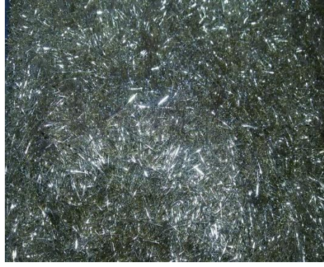
Figure 3.3. Micro steel fiber used in this study
