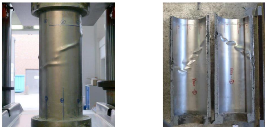
Figure 2.14 Steel-wrapped UHPC tube: test set-up (left) and cut open specimen (right) (Scholle and Lohaus, 2012)
