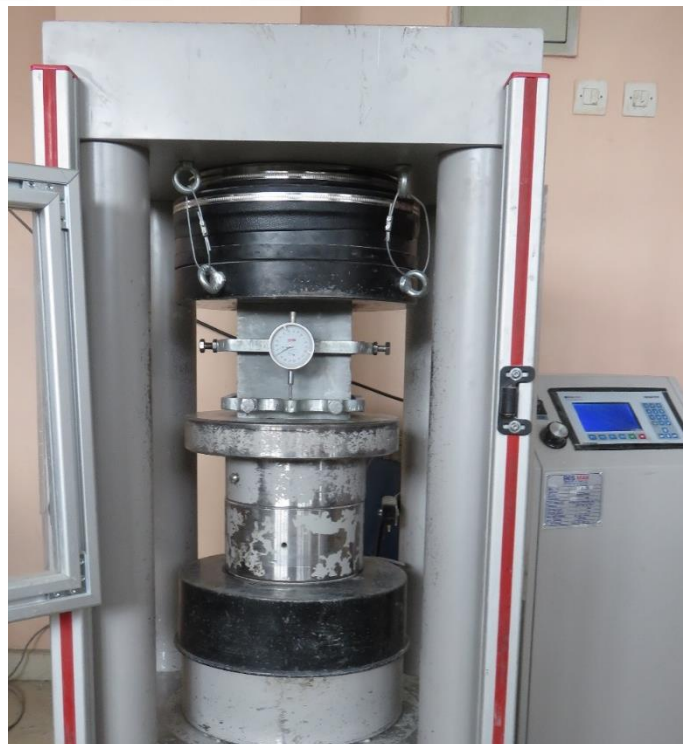
Figure 3.6 Modulus of elasticity test
