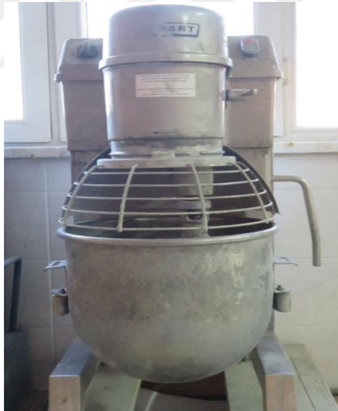
Figure 3.3 Hobart mixer used for mixing UHPC and UHPGC
