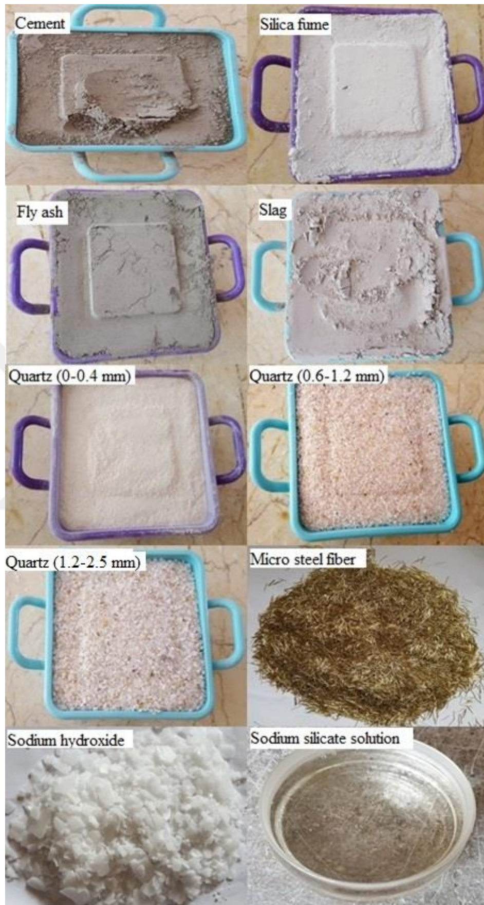
Figure 3.2 Materials to cast UHPC/UHPGC
