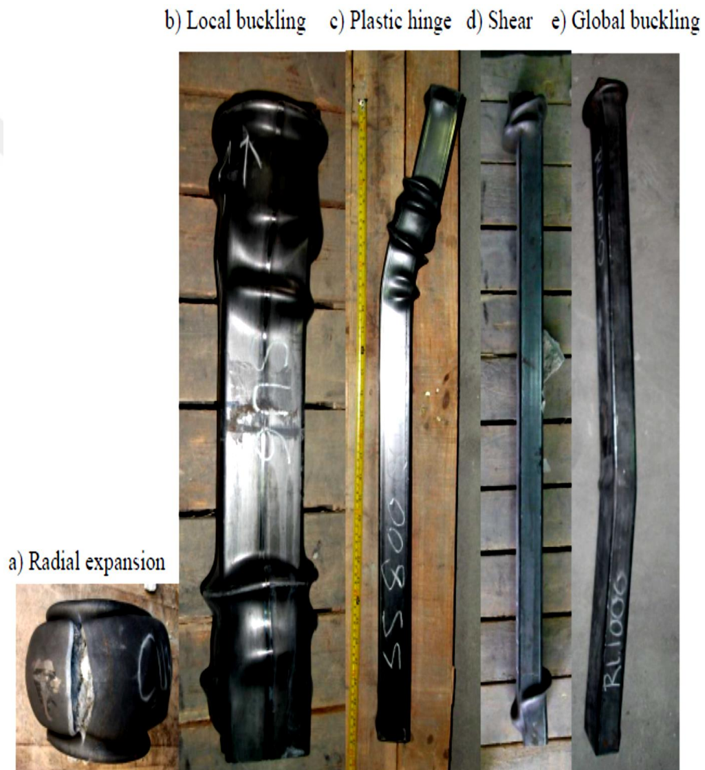
Figure 2.6 Classification of CFST column failure modes (Chu, 2014)
