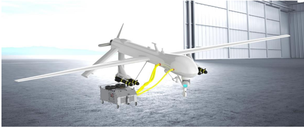
Figure 4.14 Representational image of the mobile FE-PCA unit together with the MQ-1 Predator.
