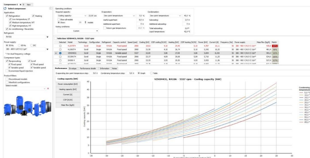
Figure 3.8 Compressor selection outputs
