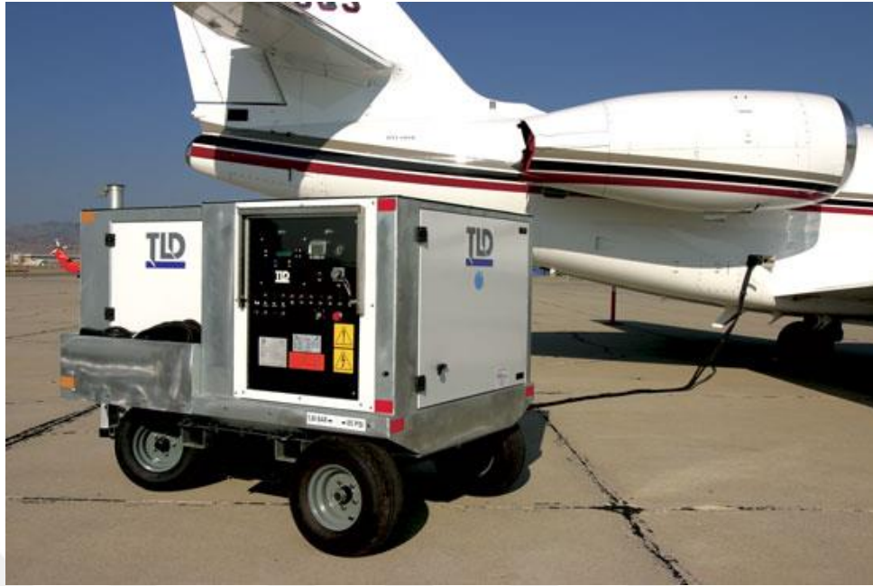
Figure 1.6 TLD GPU-28-CUP diesel ground power unit
