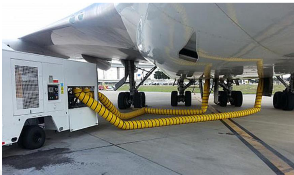
Figure 1.3 An operational view of a mobile PCA unit
