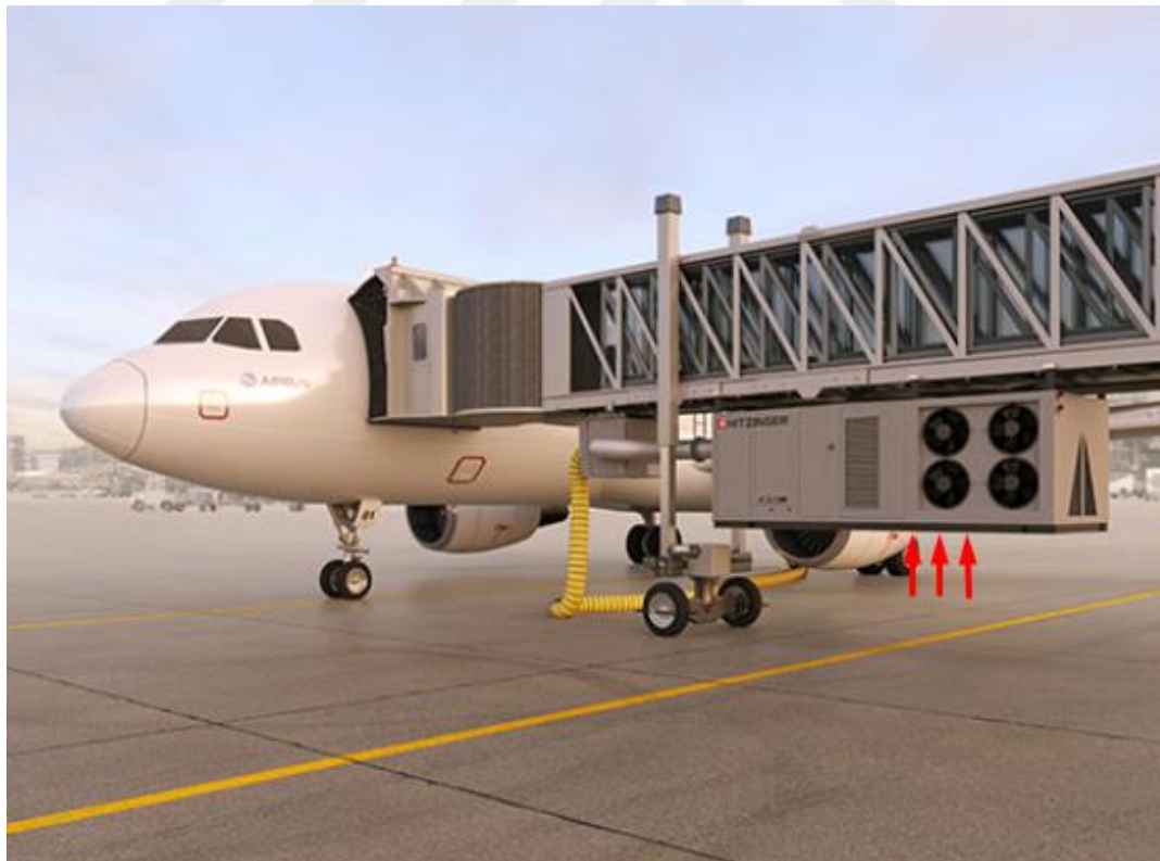
Figure 1.4 Bridge mounted PCA units generally hang under the bridge [6]
