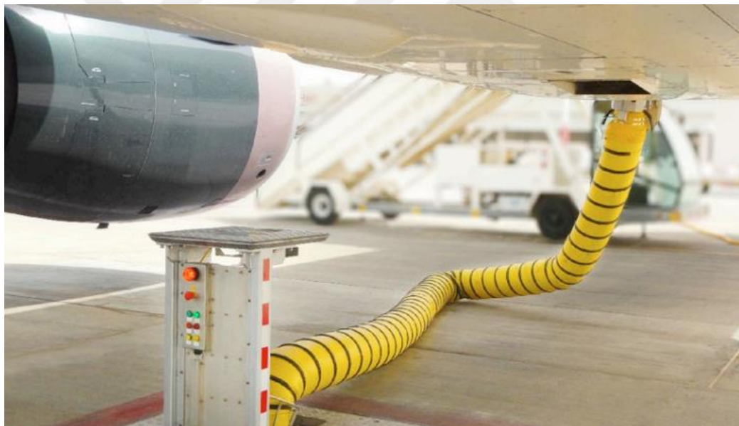
Figure 1.5 Ground-mounted PCA unit [7]
