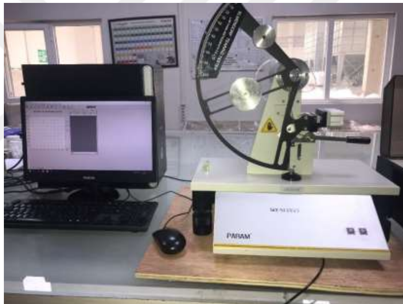
Figure 3.8 LabThink tear tester
