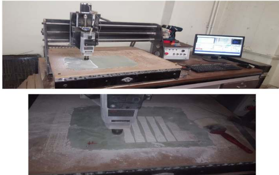
Figure 3.9 Cutting the Specimen Using CNC Machine
