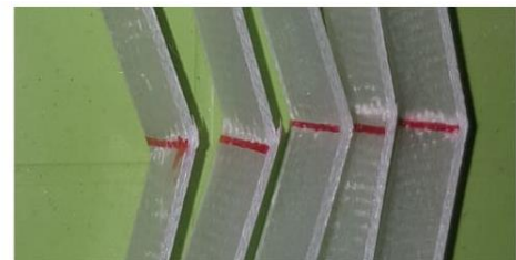
Figure 4.12 Flexural Specimens after Test
