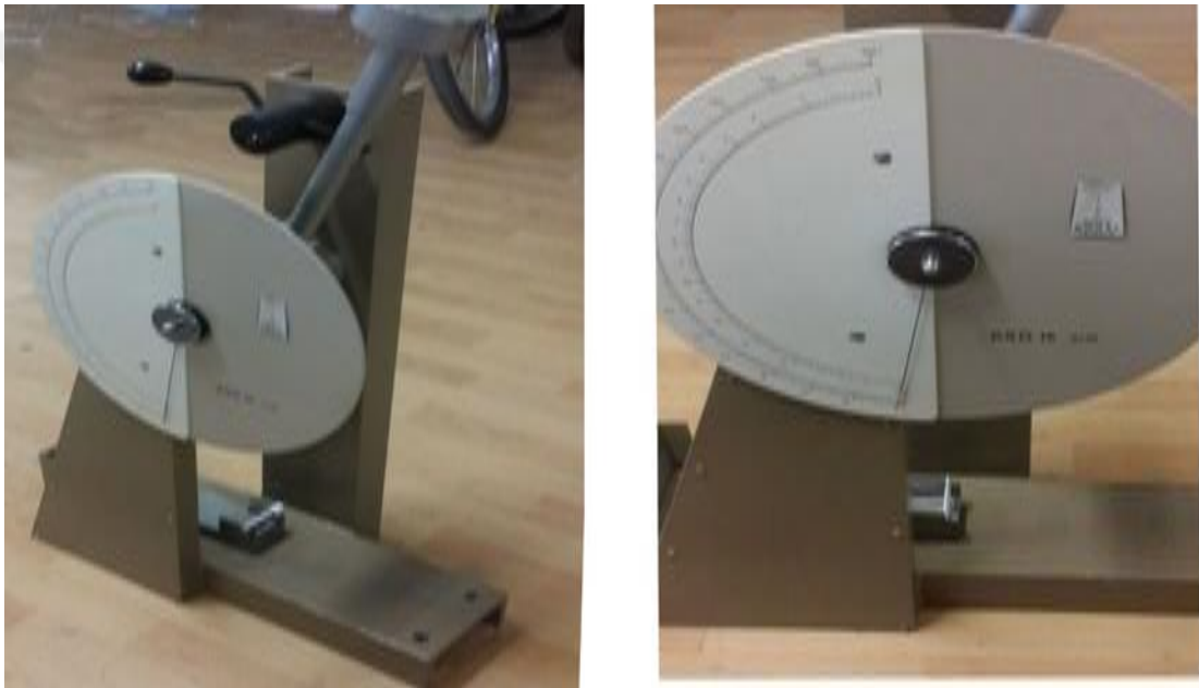
Figure 3.15 Charpy impact test (flatwise impact loadings)
