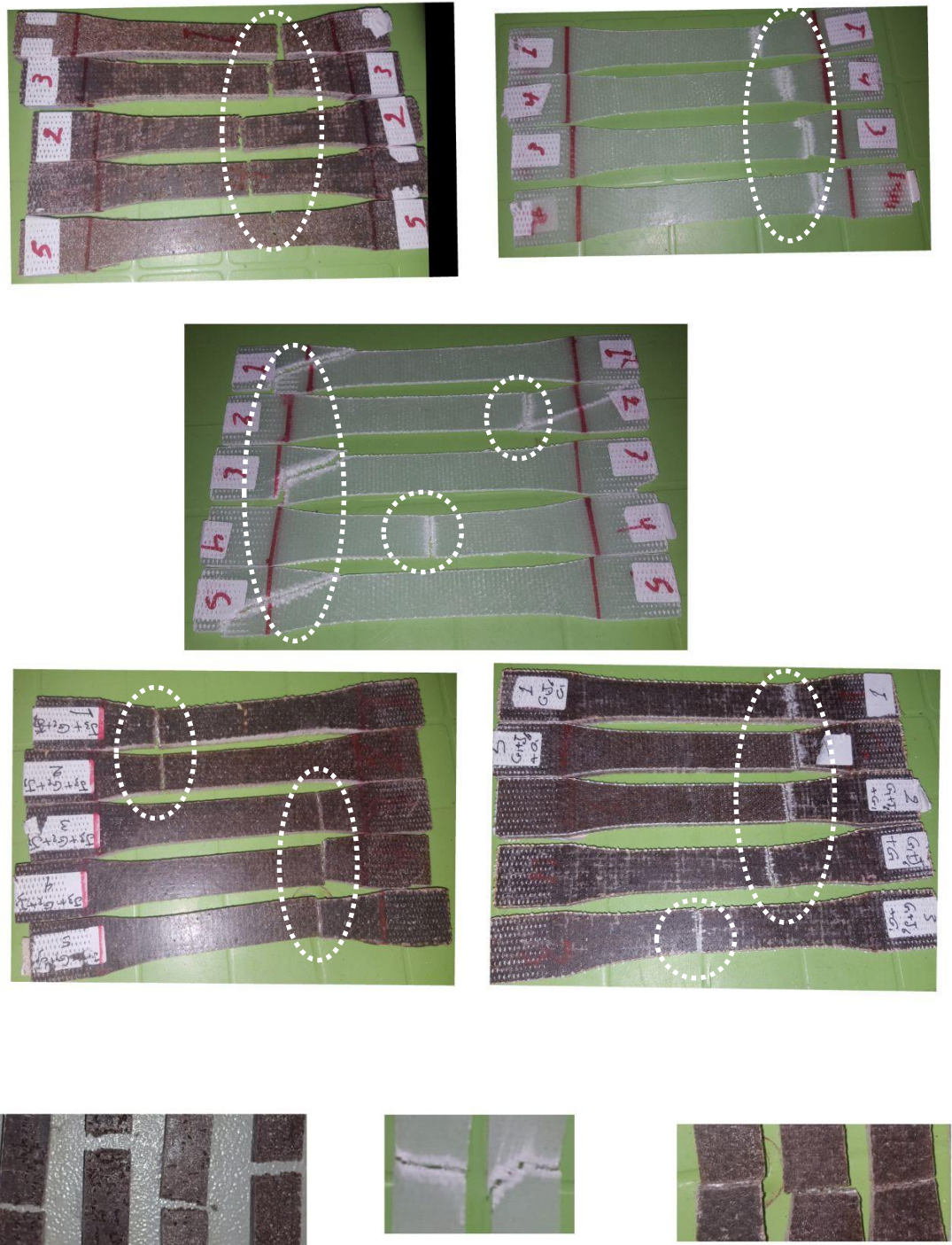
Figure 4.5 Failure Specimens of Different Composite Laminates After Tensile Test.
