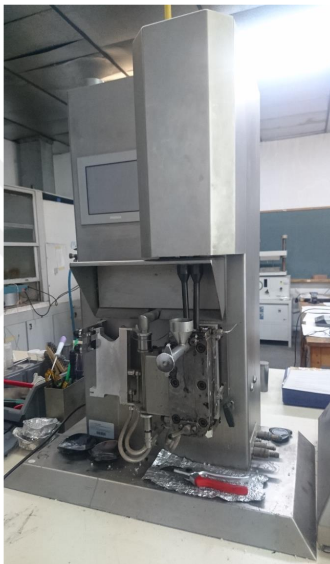
Figure 3.5. The lab-scale micro-compounder used in this study.
