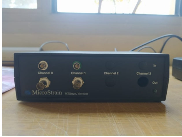
Şekil 6: Microstrain DVRT sensörü (Microstrain, Inc, Burlington, VT)
