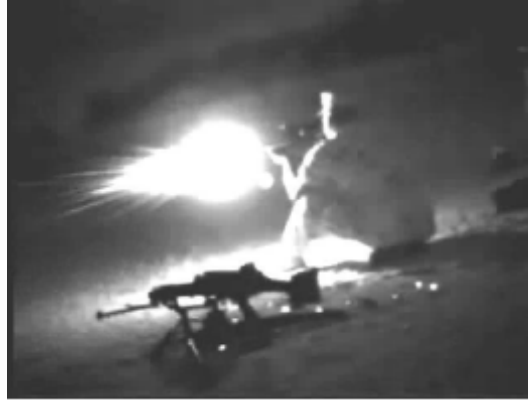
Figure 2.7: Muzzle flare detected by SWIR[18]
