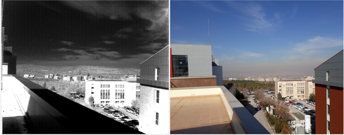
Figure 5.7: SWIR image acquired with NANOTAM SWIR Camera vs visible image captured with a smart phone camera
