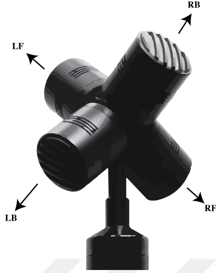
Figure 2.11: Illustration of Tetrahedral Microphone and its directions
