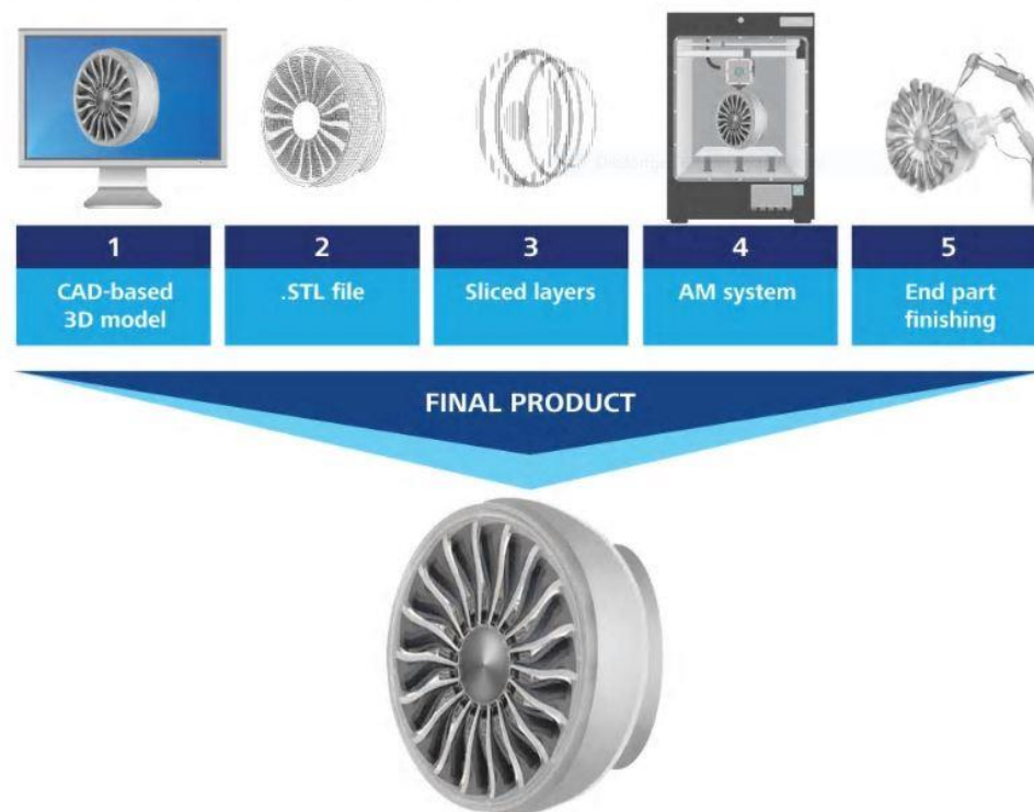
Figure 3.2 Additive manufacturing process flow [19]
