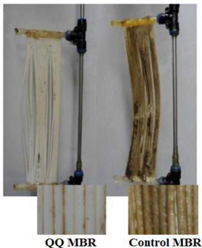
Figure 5. 10 : The appearances of the membranes of Control MBR and QQ MBR.
