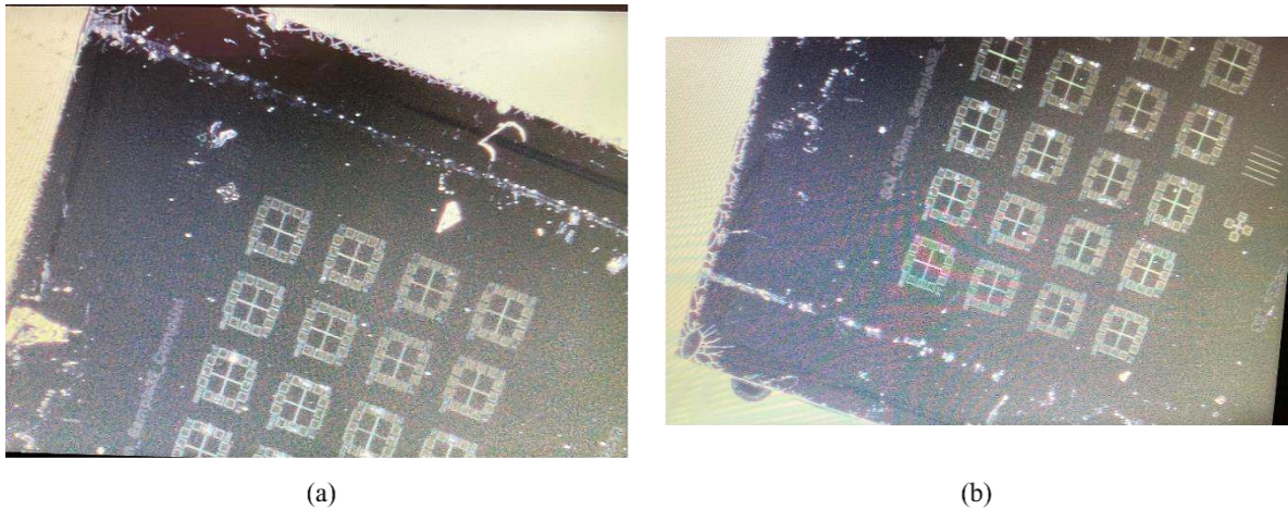
Figure 82: Marks of outer pins where force is applied on the SOI chip. (a) right end, and (b) left end of the chip, captured via optical microscope.
