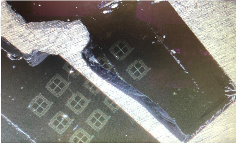
Figure 83: Micrograph of the broken SOI chip at 20\mu\text{m} pin displacement.
