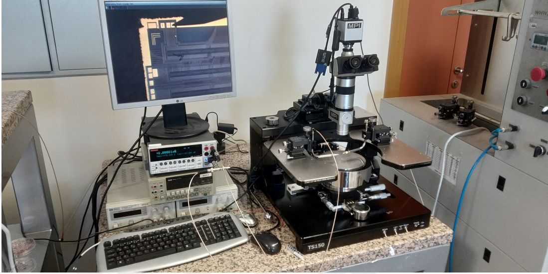
Figure 3.17: Probe station test setup showing Keithley 2400 SMU being used to test for shorts.
