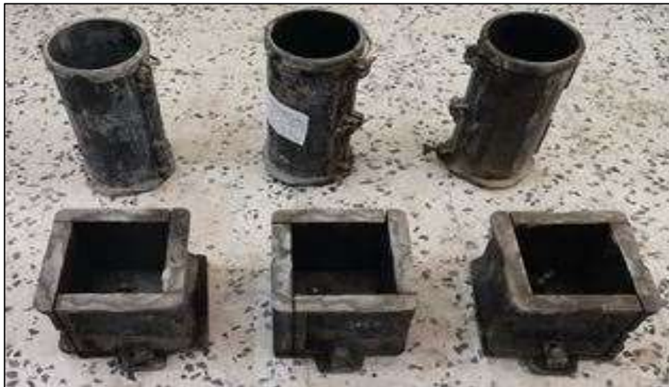
Figure 3.9: Used Concrete Moulds.
