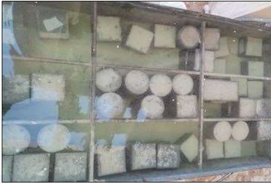
Figure 3.8: Concrete Moulds Curing Basin With Water.
