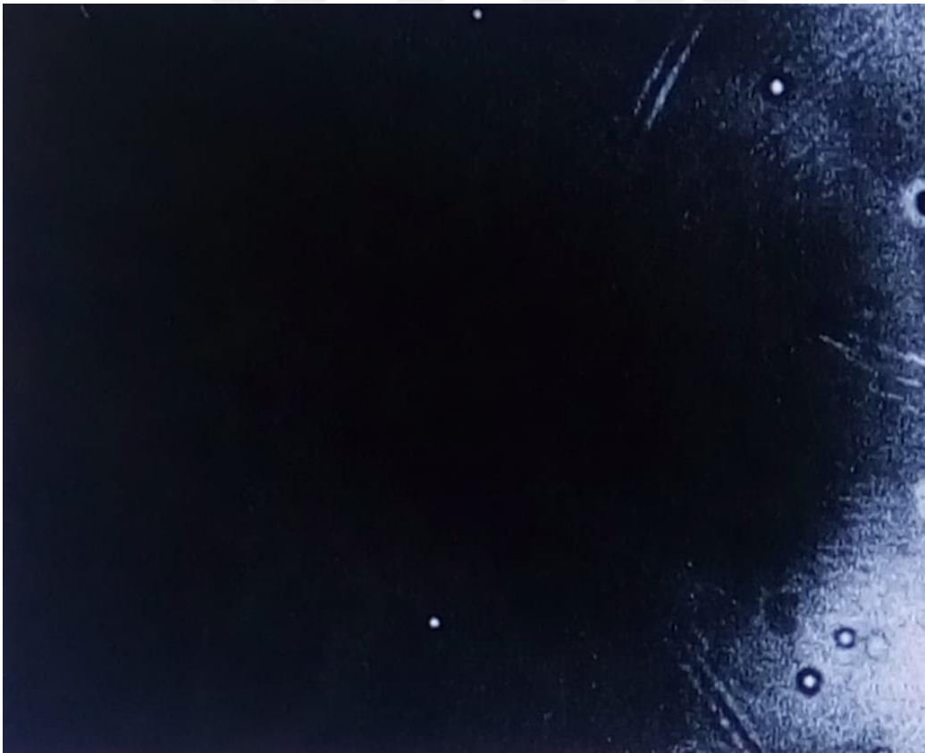
Figure 4.14. Detector image with inappropriate under-fill material
