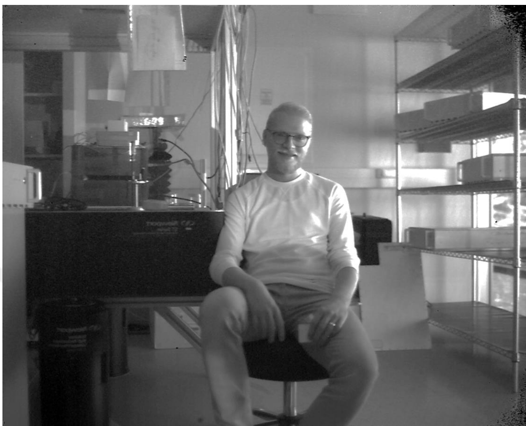
Figure 4.17. Image taken by a detector with FCB problems at two corners
