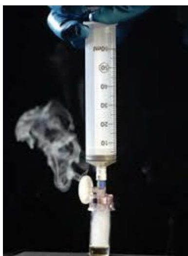
Figure 2-2: Alaris Smart Site with release of titanium smoke [7].
