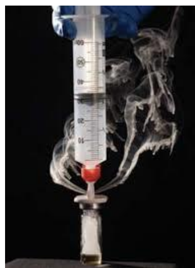
Figure 2-3: Chemo MiniSpike Plus with release of titanium smoke [7].
