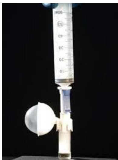
Figure 2-1: PhaSeal with no release of titanium smoke [7].
