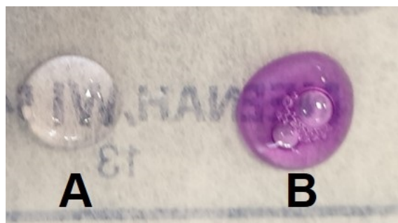
Figure 4.7: Purpald test on IgG (A) before and (B) after the oxidation reaction.
