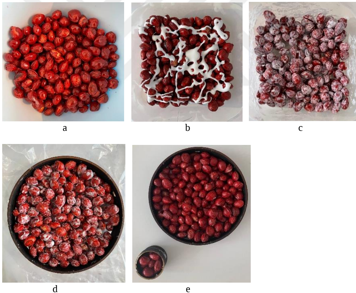
Figure 15. Preparation steps of material I: a) Painted cherry seeds b) Addition of wood glue c) Mixing wood glue and red cherry seeds d) The prepared mixture in the mold e) Mixture upon drying
