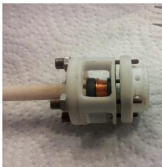
Figure 3.5. Microcantilevers mounted in a Teflon housing with an electromagnetic coil
