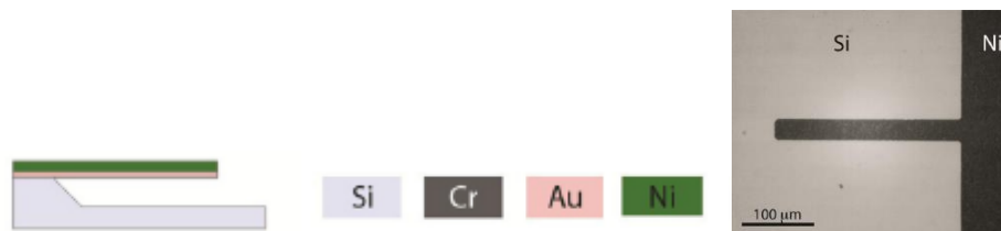
Figure 3.4. (left) Schematic representation of microcantilever used for the fluid density and viscosity measurements (right) Micrograph of the microcantilever
