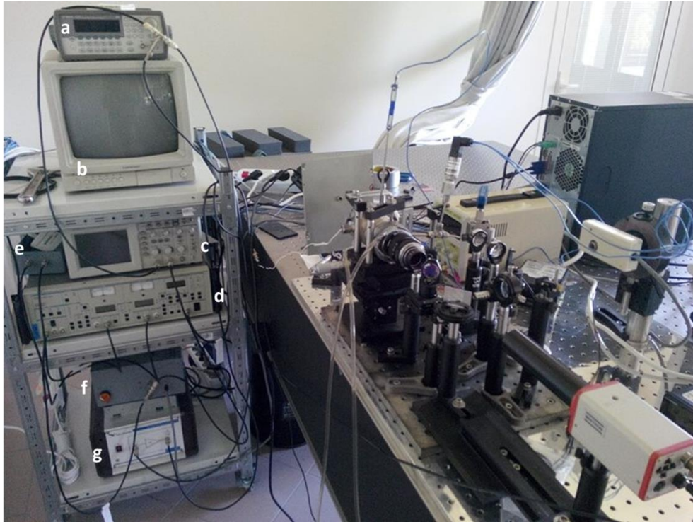
Figure 3.2: The experimental setup. Electronic Equipments (a) Agilent 33220A Arbitrary Waveform Function generator (b) Display (c) Tektronix TDS 1012 TDS 2000C Oscilloscope (d) Stanford Research Systems SR530 Dual Phase Lock in Amplifier (e) National Instruments USB 6008 Data Acquisition apparatus (f) Voltage Detection system connected to QPD (Quadrant Photodiode Detector) (g) Falco System High Voltage Amplifier WMA-300
