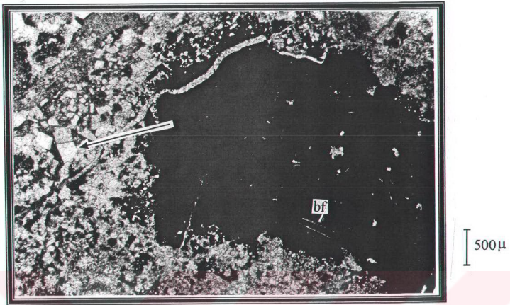
Figure 3.40. Microfacies 3, Intraclastic-Algae / Bioclastic Wackestone Yellicebelen Measured Section, No: 01/87, Güvercinlik Formation Original Texture of this Microfacies that is Composed of Small and Thin Bioclast Fragment (bf) and Dark Colored Micritic Matrix. In the Some Areas of the Microfacies 3, Well-Developed Planar-Euhedral, Planar-Subhedral and Nonolunar-Anhedral Dolomitic Crystals have Been Covered the Original Texture (Arrow).
