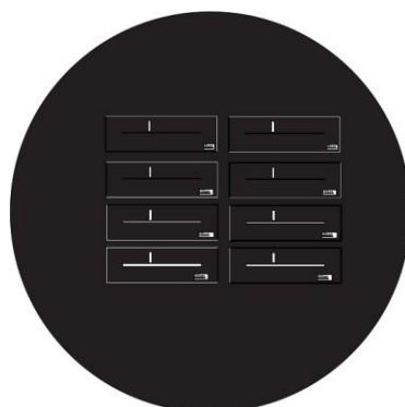
Figure 2.5 Image of the 3-inch photomask design including all different chips with different microchannel widths.
