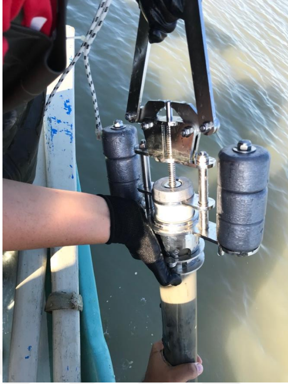
Figure 2.5: Core sampling (Photo: Ü. Nihan Tavşanoğlu, 2020).
