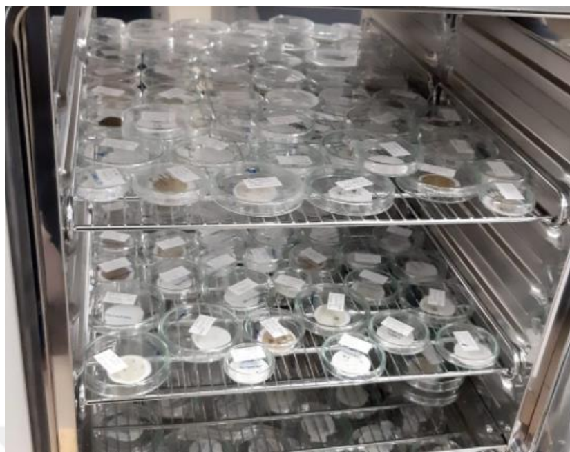
Figure 2.9: Samples arranged in the oven for drying (photo: Melike Seyfe, 2020).
