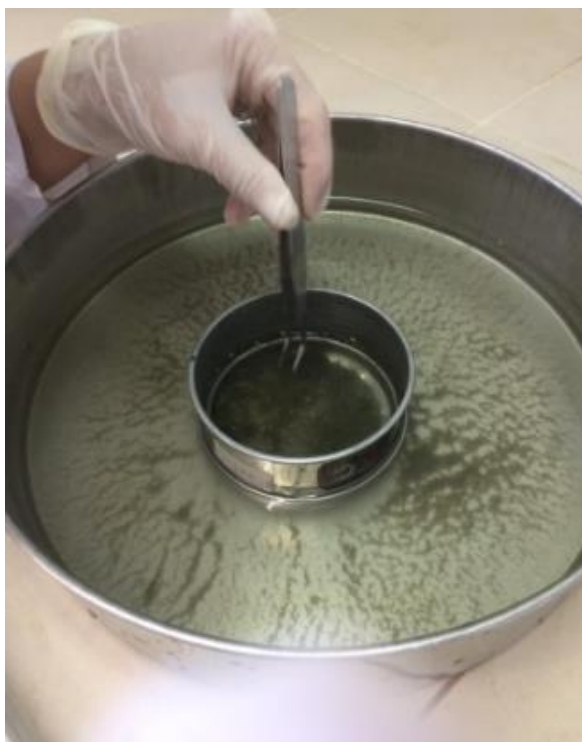
Figure 2.7: Sediment Filtration (Photo: Elif Paçal, 2020).
