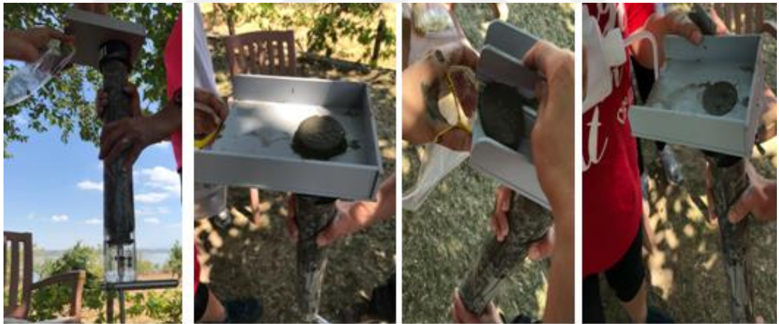
Figure 2.6: Core slicing (Photo: Ü. Nihan Tavşanoğlu, 2020).
