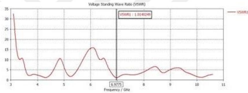
Figure 10.3: VSWR performance of the designed antenna
