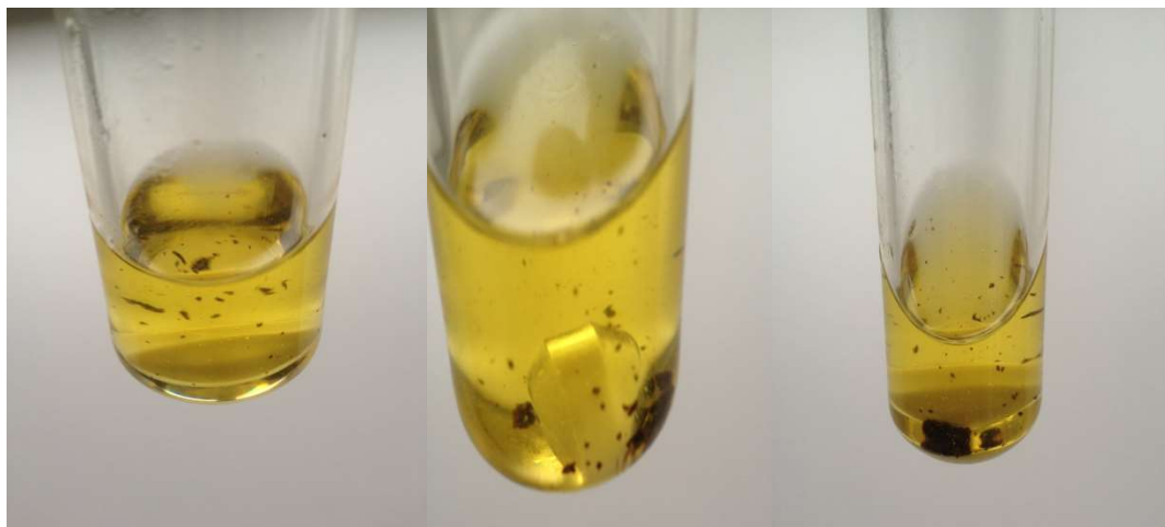
Figure 4.6 The clay dispersed in the form of flakes in oil after repetitive use
