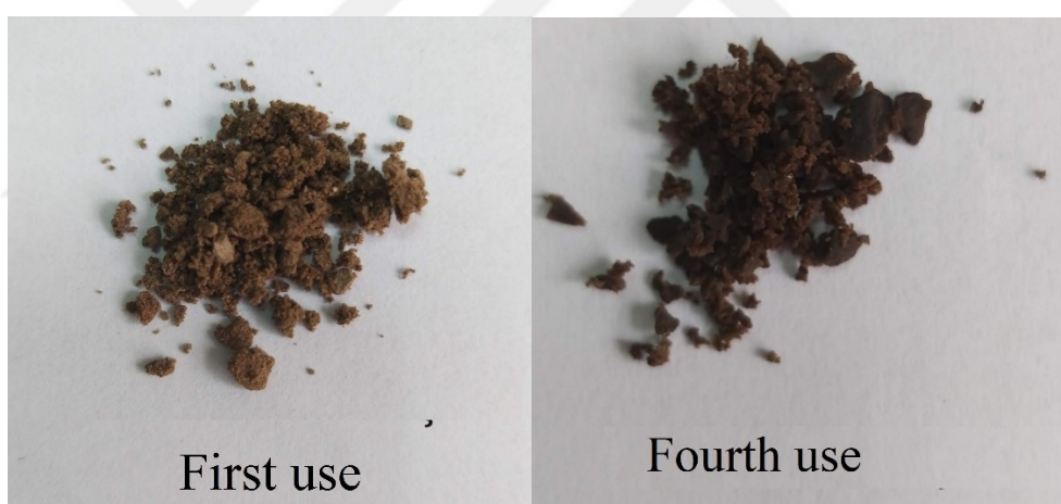
Figure 4.5 Physical structure of bleaching clay during repetitive use
