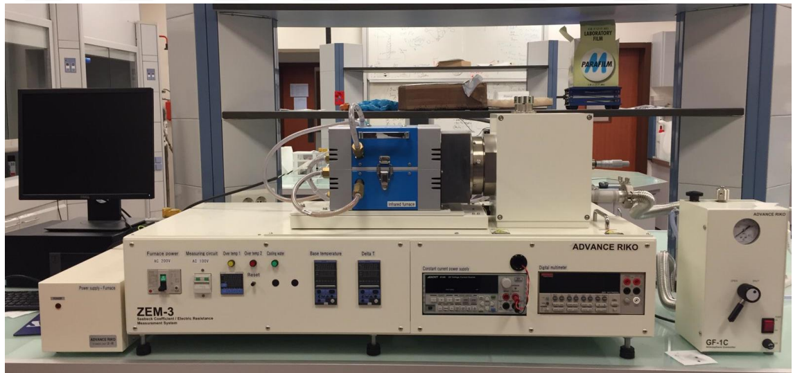
Figure 3.7 ZEM-3 Seebeck and electrical resistivity measurement system.
