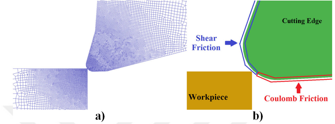
Figure 4.1: a) Modified cutting edge geometry used in finite element simulation. BUE edge radius is selected to be 2.5 \mu\text{m} . b) Hybrid friction model used in the finite element simulations.
