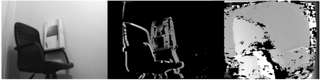
Figure 2.7 : The reference frame on the left, corresponding disparity map obtained with passive stereo (second) and active stereo (third).
