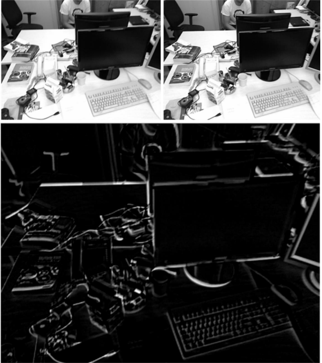
Figure 3.3 : Reference and source camera frame (top), related intensity image (bottom).
