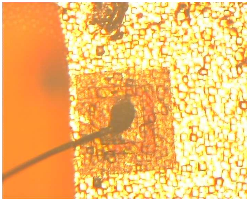
Figure 5.16: Photograph taken during ball bonding process for the unpolished surface.
