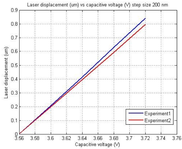
Figure 4.16: Laser displacement vs capacitive sensor voltage step size 200nm
