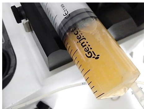
Figure 5.1. Bubbles formed inside anolyte supply syringe.
