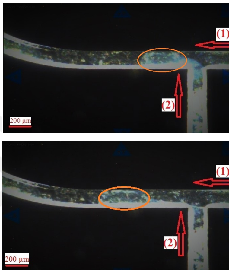
Figure 3.6: Droplet generation images at the T-junction. Arrow 1 shows the flow direction of NMF as the carrier fluid with a flow rate of 9.5 \mu\text{L}/\text{min} . Arrow 2 indicates the direction of reagents with a total flow rate of 4.0 \mu\text{L}/\text{min} .
