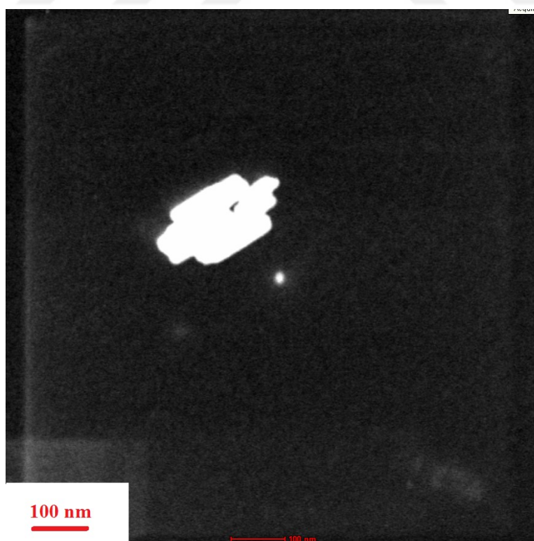
Figure 4.15: TEM results of the silica encapsulation of quantum dots: Experiment 4.3 at 50 °. Quantum dot nanoparticles could not be detected while the silica clusters indicate the particle agglomeration.
