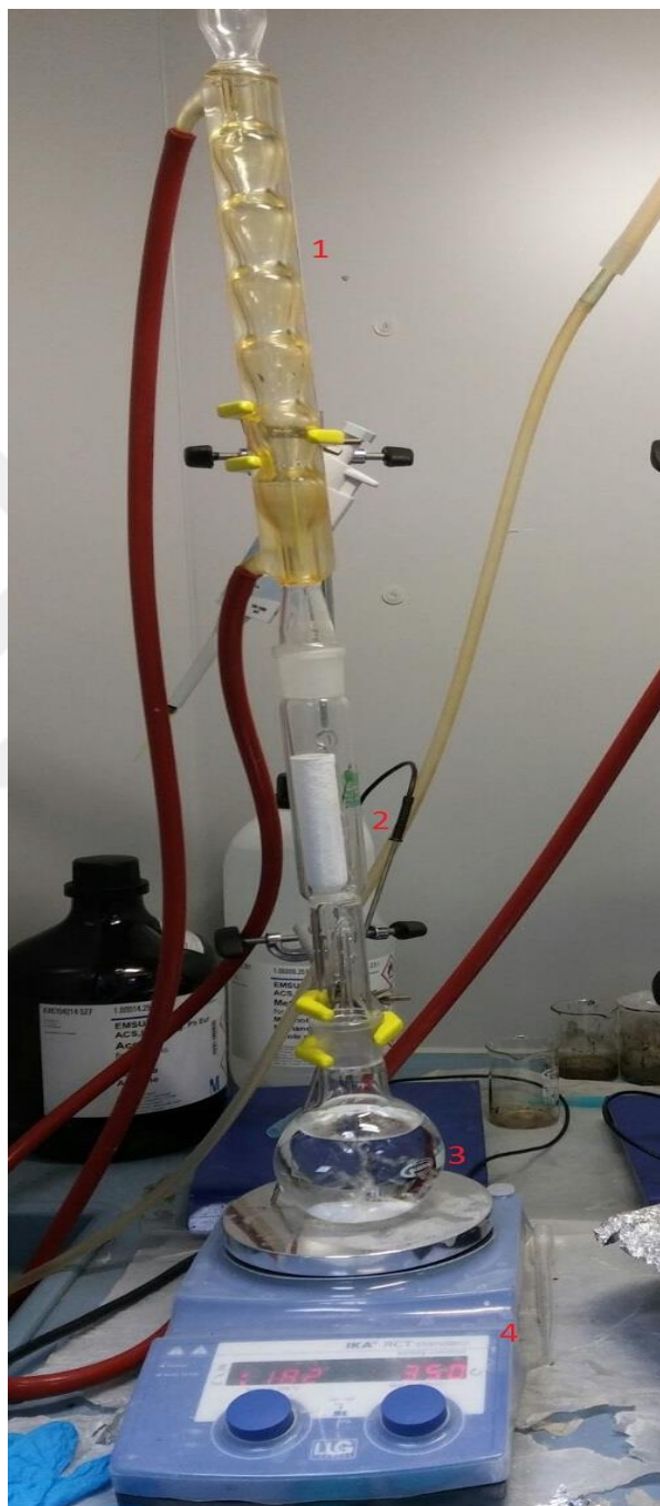
Figure 10: Soxhlet Extraction Experimental Setup (1. Condenser, 2. Extraction thimble, 3. Solvent, 4. Heater)
