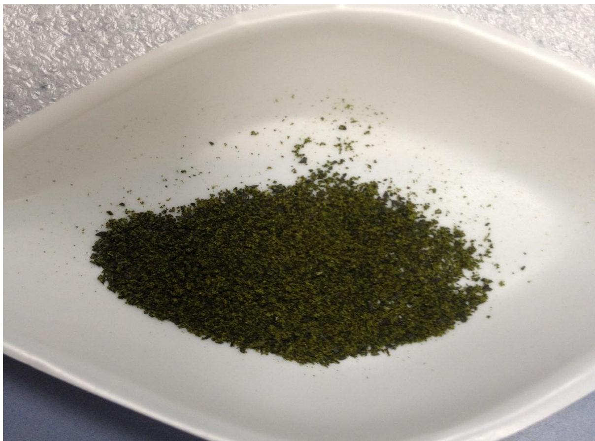
Figure 9: Microalgae powder obtained after grinding with liquid nitrogen
